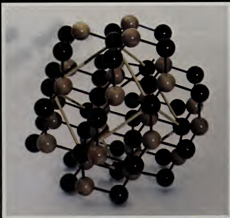
B. Model of the diamond crystal lattice. All atoms represent carbon; the black and tan spheres show alternating planes made up of chair cyclohexane rings.
