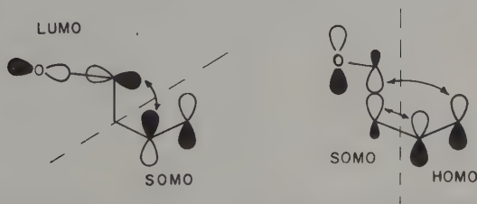
Fig. 46. Frontier orbital interactions controlling reactions of triplet ( \pi\pi^* ) and singlet ( n\pi^* ) states of \beta,\gamma -unsaturated carbonyl compounds.
