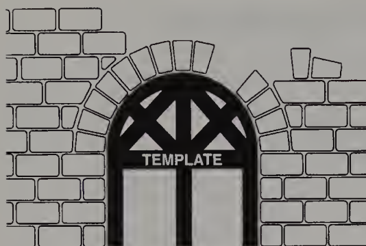
Figure 1-2 The template (in black) is used to hold stone blocks in place while they are cemented together; the template is removed from the finished archway.
