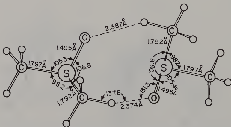
FIGURE 47. \text{CH}_3\text{S}(\text{O})\text{CH}_3 dimer I, structure 111 in Tables 28-30
