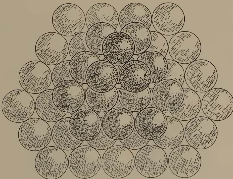
FIG. 11-4.—The arrangement of spheres in hexagonal closest packing.
