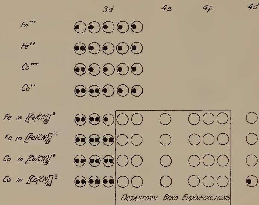
FIG. 5-3.—Occupancy of orbitals by electrons in hypoligating and hyperligating octahedral complexes of bipoisitive and tri-positive iron and cobalt.
