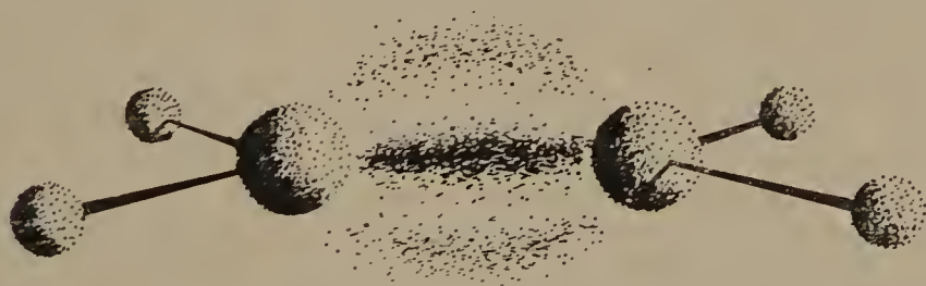
FIG. 4-9.—A representation of the ethylene molecule with the double bond shown as a sigma bond and a pi bond.
