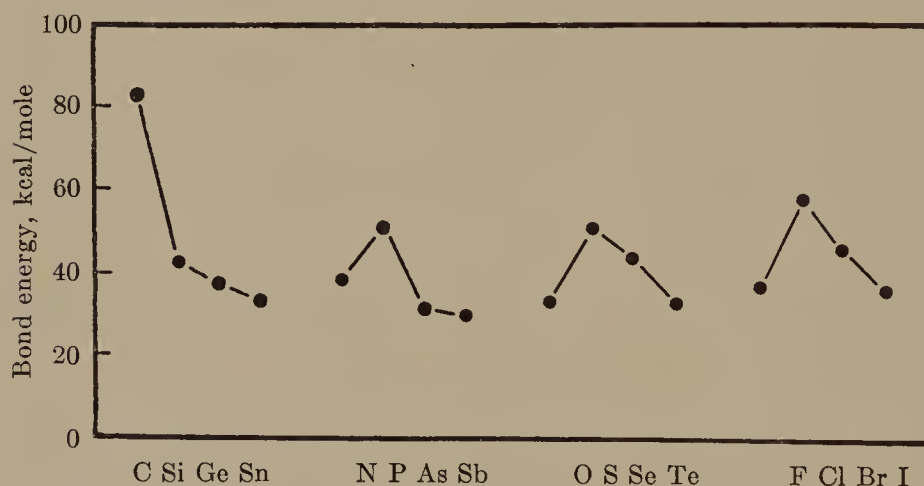
FIG. 3-6.—The values of single-bond energies of elements.
