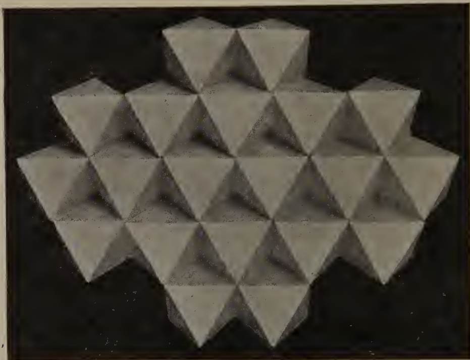
FIG. 7-10.—Layers of octahedra corresponding to the composition MX_2 . There is an atom M in the center of each octahedron, and an atom X at each octahedron corner, shared by three octahedra. The layer is to be considered as extending to infinity.
