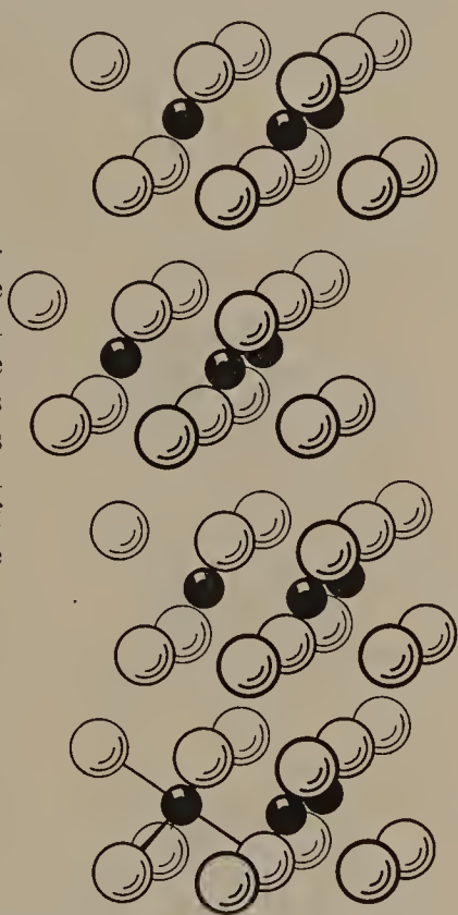
FIG. 7-11.—The arrangement of cadmium atoms (small circles) and chlorine atoms (large circles) in the rhombohedral crystal cadmium chloride, \text{CdCl}_2 . The atoms are arranged in octahedral layers, as represented in Figure 7-10. These layers are superimposed in the manner indicated in the figure. Repetition in the direction of the trigonal axis (vertical) occurs after three layers.
