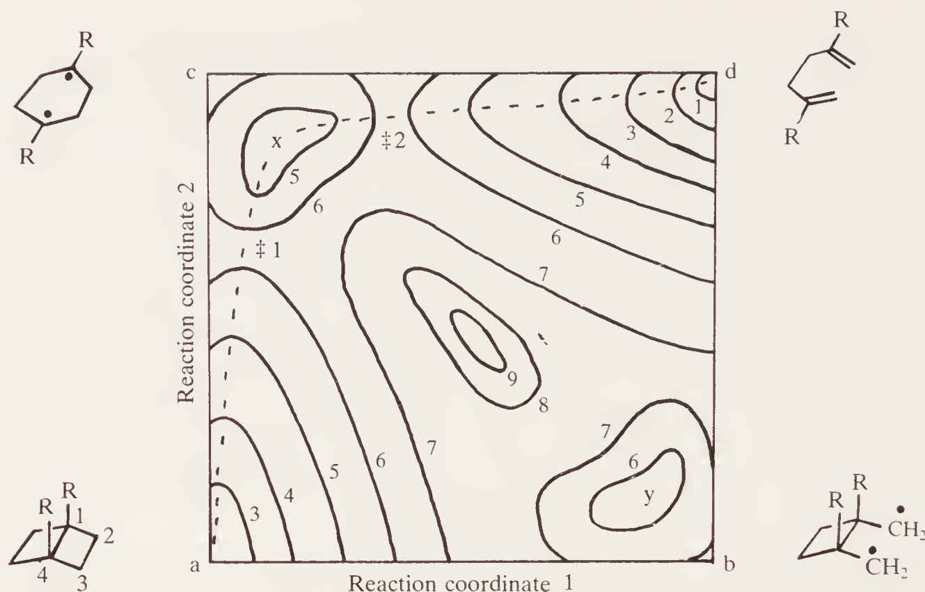
Fig. 10.2. Molecular potential-energy reaction map for the isomerization of a bicyclo[2.2.0]hexane into a hexa-1,5-diene. (Increasing numbers indicate contours of increasing potential energy.)
