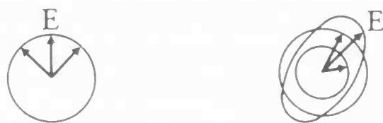
Figure 8.17 Left plane polarized lights; right elliptically polarized light produced from plane polarized light by differential absorption.
