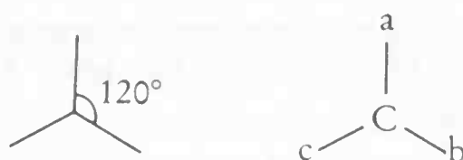
Figure 1.2 Trigonal geometry for \text{Cabc} with 120^\circ bond angles.
