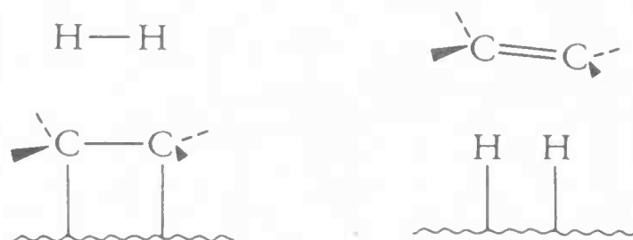
Figure 12.7 Coordination of alkenes and hydrogen to metal surfaces results in catalysis of syn additions.
