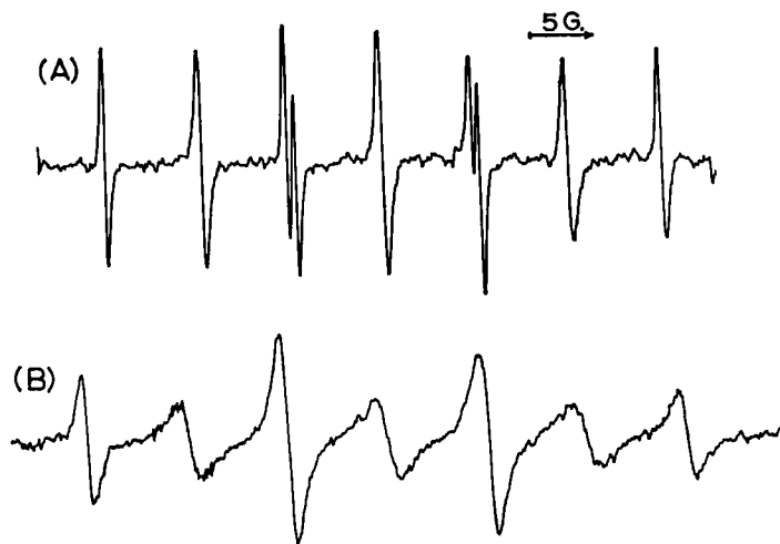
Fig. 2. The esr spectra of (A) the nitroxide of tritylglycine methyl ester in dioxane and (B) tritylglycine in aqueous sodium hydroxide (pH 8) at room temperature. Courtesy of American Chemical Society, taken from J. Org. Chem. , 34 , 4072 (1969).
