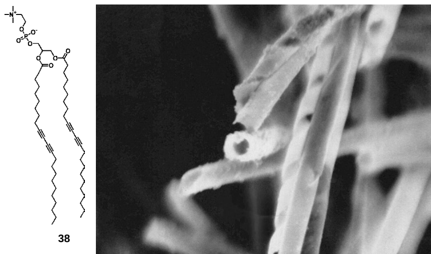
Figure 5.27 Scanning electron micrograph of copper-coated DC 8,9 PC ( 38 ) tubules. Tubules are hollow with diameter of approximately 0.5 \mu\text{m} (bar = 0.5 \mu\text{m} ). Helical wrappings evident in some tubules are all right handed. Reprinted with permission from Ref. 125. Copyright 1998 by the American Chemical Society.
