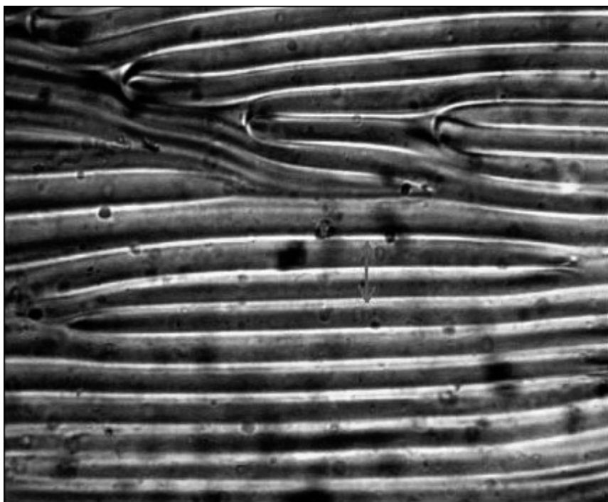
Figure 7.6 Fingerprint texture of lyotropic cholesteric: double-headed arrow corresponds to pitch.
