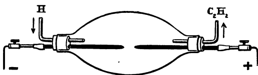
FIG. 40.—Formation of Acetylene from Carbon and Hydrogen.
