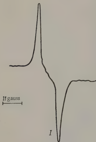
FIGURE 9. EPR spectrum of the mixture of alkylaluminum compounds with Ti(C_5H_5)_2X_2 in toluene (equimolar ratio of Al to Ti; reagent concentration less than 1 \cdot 10^{-3} mole/liter).
