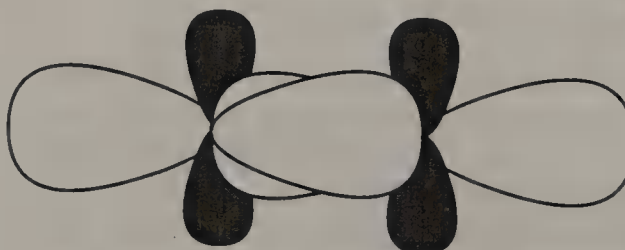
schematic view of the \langle d_{z^2} | d_{z^2} \rangle overlap at short M-M distance
