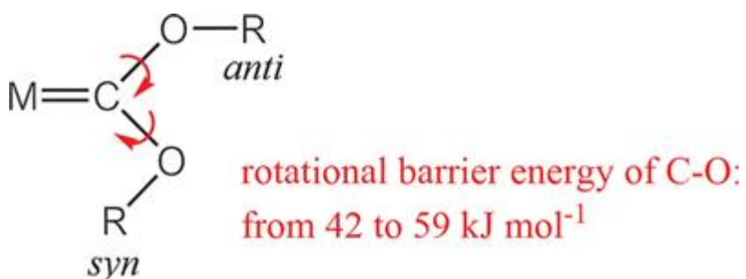
Figure 5.6 Syn/anti structure of a Fischer carbene complex.
