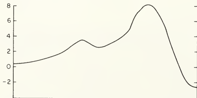
Fig. 1-9. Cross section of minimum energy through Fig. 1-8, the conventional plot of energy versus reaction coordinate.
