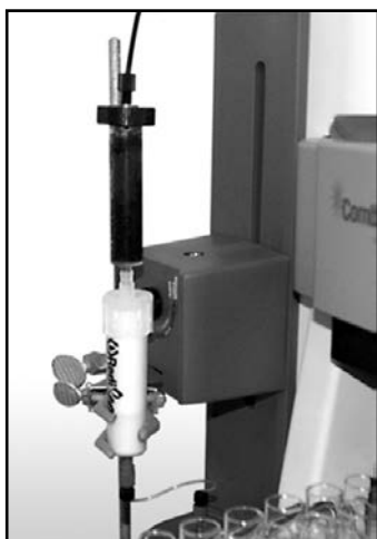
Figure 28: Photo of solid load cartridge connected to column to bypass valves in the instrument
