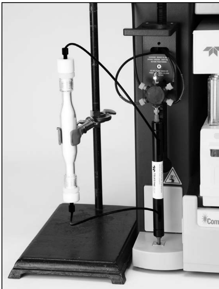
Figure 98: Photo of column mount part number 60-5394-432 (shown below valve) used to adapt a CHP-20 column to a CombiFlash Rf system.
