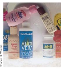
Some common products packaged in high-density polyethylene containers.
