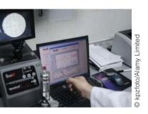
A Beckman Coulter DU 800 infrared spectrophotometer. Spectra are shown in the monitor.
