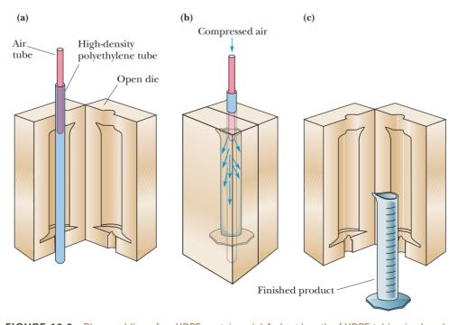
**FIGURE 16.6** Blow molding of an HDPE container. (a) A short length of HDPE tubing is placed in an open die, and the die is closed, sealing the bottom of the tube. (b) Compressed air is forced into the hot polyethylene–die assembly, and the tubing is literally blown up to take the shape of the mold. (c) After cooling, the die is opened, and there is the container!
