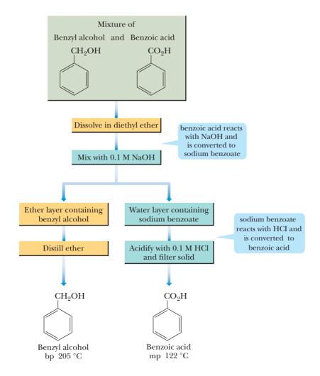
**FIGURE 13.1** Flowchart for separation of benzoic acid from benzyl alcohol.
