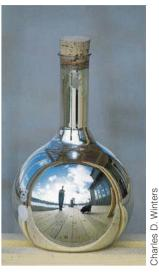
A silver mirror has been deposited in the inside of this flask by the reaction of an aldehyde with Tollens' reagent.
