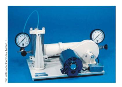
A Parr shaker-type hydrogenation apparatus allows chemists to achieve gas pressures up to 100 atm.
