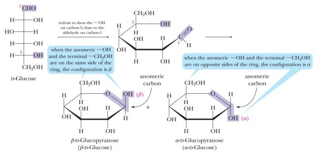
**FIGURE 17.1** Haworth projections for  $\beta$ -D-glucopyranose and  $\alpha$ -D-glucopyranose.
