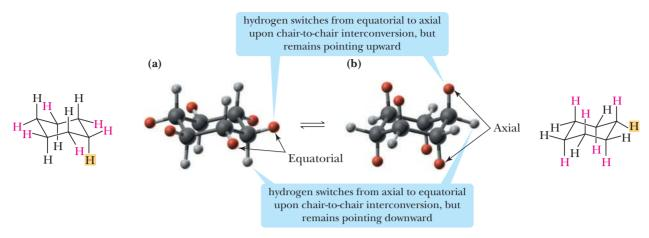
FIGURE 3.10 Interconversion of chair cyclohexanes. All C—H bonds that are equatorial in one chair are axial in the alternative chair, and vice versa.
