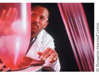
Polyethylene films are produced by extruding the molten plastic through a ring-like gap and inflating the film into a balloon.
