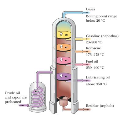
FIGURE 3.13 Fractional distillation of petroleum. The lighter, more volatile fractions are removed from higher up the column and the heavier, less volatile fractions from lower down.
