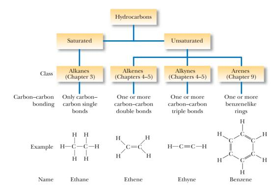
FIGURE 3.1 The four classes of hydrocarbons.
