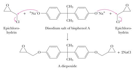
To prepare the following epoxy resin, the diepoxide monomer is treated with 1,2-ethanediamine (ethylene diamine):
