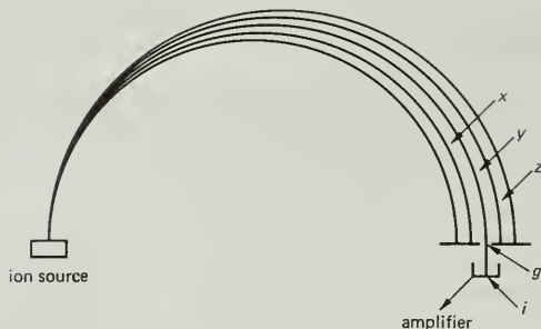
FIGURE 16.2 Ions with m/e = y are focused on the collector i through slit g .
