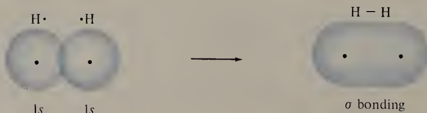
FIGURE 1.7 When the 1s atomic orbitals of two hydrogen atoms overlap, a bonding molecular orbital results.
