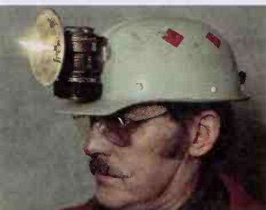
The light of one kind of head-lamp used by miners and cave explorers is given off by the combustion of acetylene, which is produced by the slow addition of water to calcium carbide. (Charles D. Winters)
