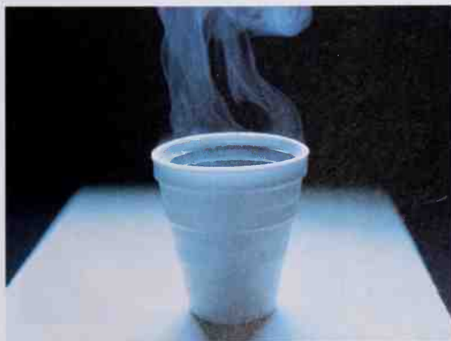
The low thermal conductivity of polystyrene makes it a good insulating material. ( Charles D. Winters )
