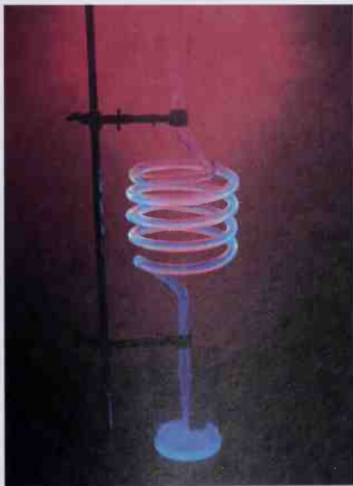
Chemical reactions often release energy. The reaction in this tube and beaker releases energy in the form of light in a process called chemiluminescence. (Charles D. Winters)
