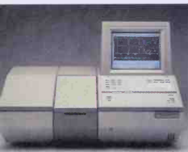
A Perkin-Elmer Paragon 1000 Fourier Transform infrared spectrometer. Infrared spectra are shown on the monitor. (Courtesy of the Perkin-Elmer Corporation)
