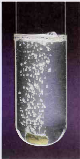
Sodium metal dissolves in methanol with evolution of hydrogen gas. (Charles D. Winters)
