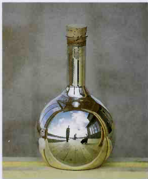
A silver mirror has been deposited in the inside of this flask. (Charles D. Winters)
