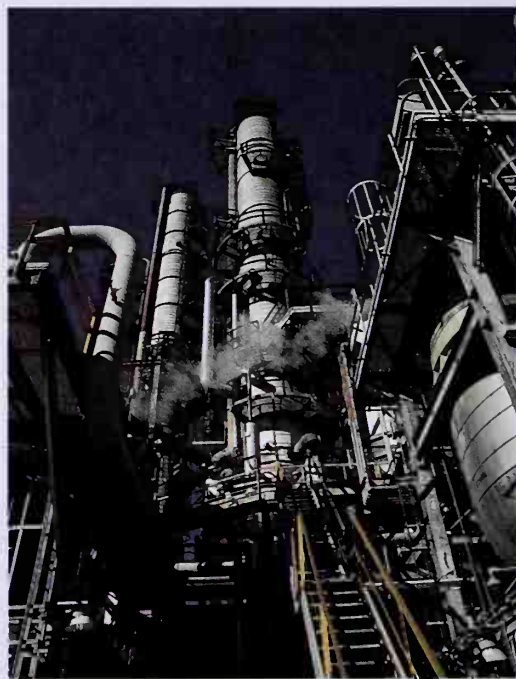
A plant for the production of acetic acid from methanol and carbon monoxide. (Courtesy of B. P. America)
