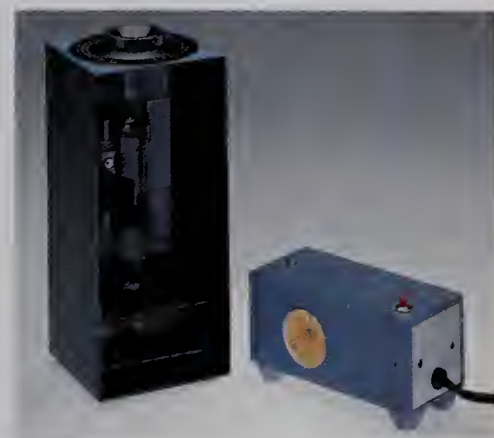
A polarimeter is used to measure the rotation of plane-polarized light as it passes through a sample. (Richard Megna, 1992, Fundamental Photographs )
