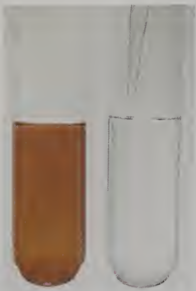
A solution of \text{Br}_2 in carbon tetrachloride is red. Add a few drops of an alkene and the color disappears. (Charles D. Winters)
