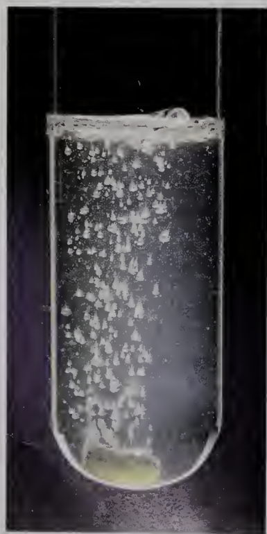
Sodium metal reacts with methanol with the evolution of hydrogen gas. (Charles D Winters)
