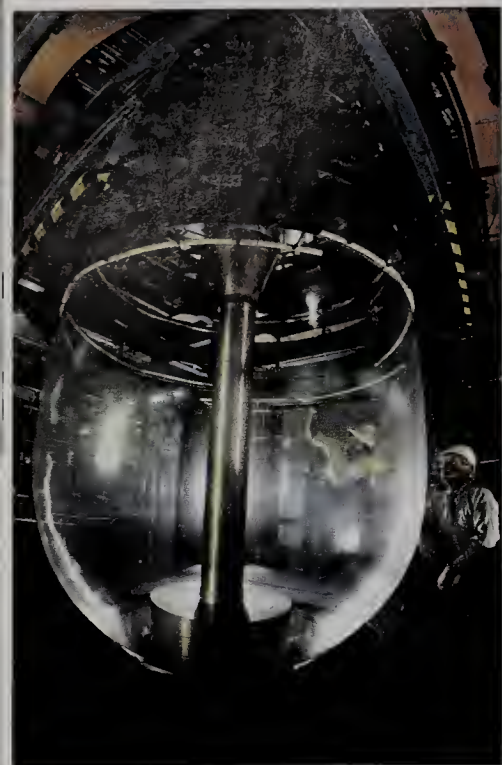
Polyethylene films are produced by extruding the molten plastic through a ring-like gap and inflating the film into a balloon. ( The Stock Market )
