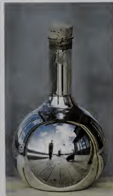
A silver mirror has been deposited on the inside of this flask by the reaction of an aldehyde with Tollens' reagent. (Charles D. Winters)
