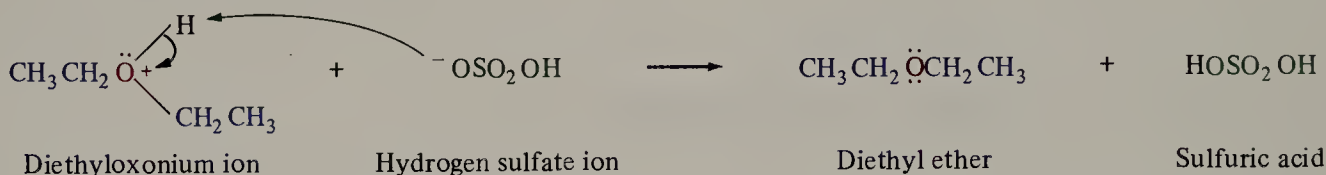
FIGURE 15.2 Sequence of steps that describes the mechanism of acid-catalyzed formation of diethyl ether from ethyl alcohol.
