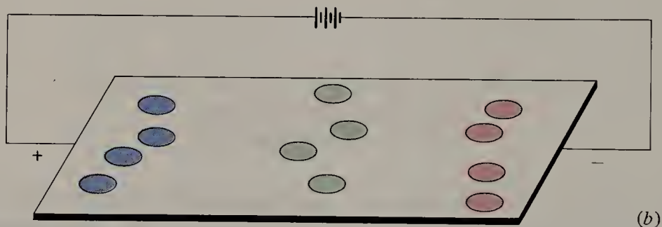
FIGURE 27.2 Application of electrophoresis to the separation of aspartic acid, alanine, and lysine according to their charge type at a pH corresponding to the isoelectric point ( pI ) of alanine.
