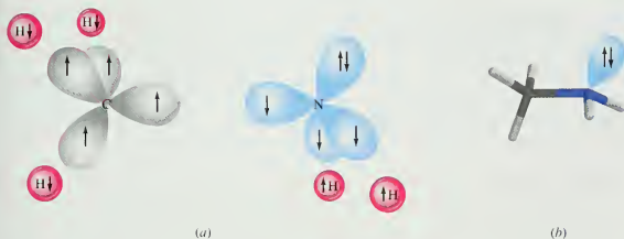
FIGURE 22.2 Orbital hybridization description of bonding in methylamine. (a) Carbon has four valence electrons; each of four equivalent sp^3 -hybridized orbitals contains one electron. Nitrogen has five valence electrons. Three of its sp^3 hybrid orbitals contain one electron each; the fourth sp^3 hybrid orbital contains two electrons. (b) Nitrogen and carbon are connected by a \sigma bond in methylamine. This \sigma bond is formed by overlap of an sp^3 hybrid orbital on each atom. The five hydrogen atoms of methylamine are joined to carbon and nitrogen by \sigma bonds. The two remaining electrons of nitrogen occupy an sp^3 -hybridized orbital.
