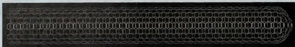
FIGURE 11.7 A portion of a nanotube. The closed end is one half of a buckyball. The main length cannot close as long as all of the rings are hexagons.
