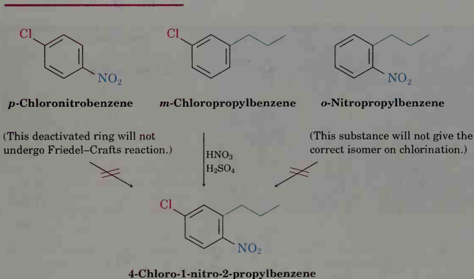
Figure 16.21 Possible routes for the synthesis of 4-chloro-1-nitro-2-propylbenzene.
