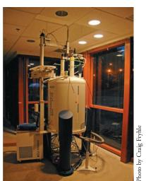
The superconducting magnet of an FTNMR spectrometer.
