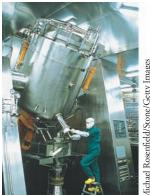
An industrial-scale reactor for preparation of an antibiotic.
