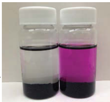
FIGURE 11.4 When \text{KMnO}_4 is added to toluene, it does not dissolve as the colorless liquid and solid indicate in the vial on the left, but as soon as some 18-C-6 is added, some \text{KMnO}_4 dissolves, as indicated by the purple color of the solution on the right.
