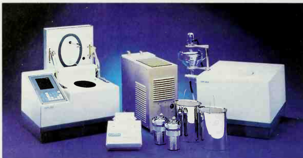
A bomb calorimeter apparatus, such as shown here, is used to precisely measure the amount of heat released upon combustion of a known amount of sample inside a sturdy metal 'bomb' (two are shown at center, front) that has been pressurized with oxygen gas.
