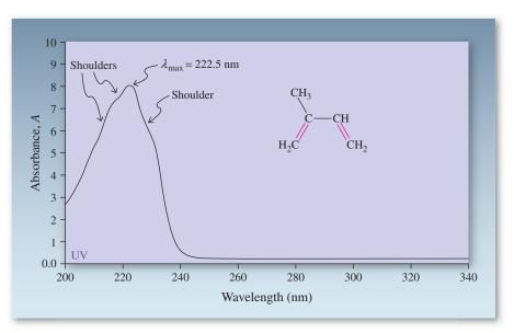
**Figure 14-15** Ultraviolet spectrum of 2-methyl-1,3-butadiene in methanol,  $\lambda_{\text{max}} = 222.5$  nm ( $\epsilon = 10,800$ ). The indentations at the sides of the main peak are called shoulders.
