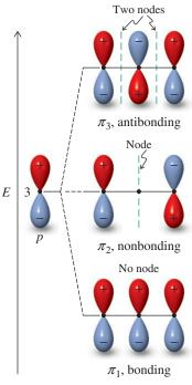
**Figure 14-2** The three  $\pi$  molecular orbitals of 2-propenyl (allyl), obtained by combining three adjacent atomic p orbitals. Note the drop in energy of the bonding molecular orbital  $\pi_1$ , reflecting the increased stability of the system. Molecular orbital  $\pi_2$  remains at the same level as the starting p orbitals and is therefore called a nonbonding molecular orbital.
