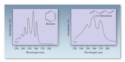
**Figure 15-6** The distinctive ultraviolet spectra of benzene:  $\lambda_{\text{max}}(\epsilon) = 234(30)$ , 238(50), 243(100), 249(190), 255(220), 261(150) nm; and 1,3,5-hexatriene:  $\lambda_{max}(\epsilon) = 247(33,900)$ , 258(43,700), 268(36,300) nm. The extinction coefficients  $\epsilon$  of the absorptions of 1,3,5-hexatriene are very much larger than those of benzene; therefore the spectrum at the right was taken at lower concentration.
