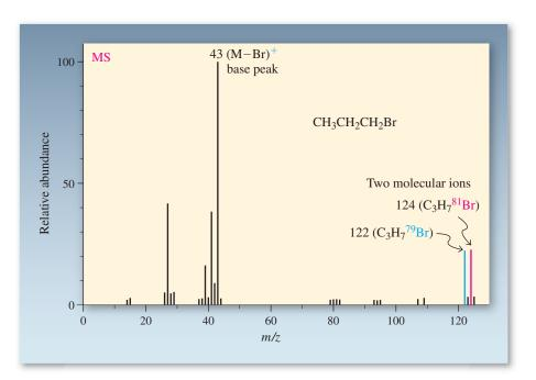
**Figure 11-24** Mass spectrum of 1-bromopropane. Note the nearly equal heights of the peaks at m/z = 122 and 124, owing to the almost equal abundances of the two bromine isotopes.
