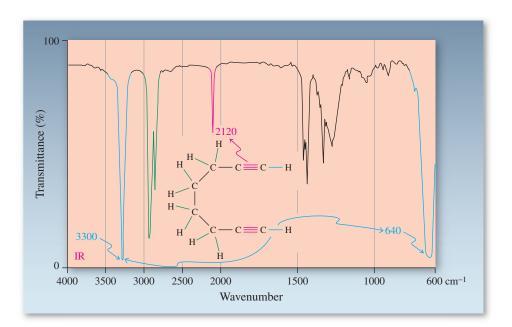
**Figure 13-6** IR spectrum of 1,7-octadiyne:  $\tilde{\nu}_{\text{Csp-H stretch}} = 3300 \text{ cm}^{-1};$   $\tilde{\nu}_{\text{C}\equiv\text{C stretch}} = 2120 \text{ cm}^{-1};$   $\tilde{\nu}_{\text{Csp-H bend}} = 640 \text{ cm}^{-1}.$
