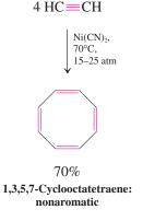
**Figure 15-17** The molecular structure of 1,3,5,7-cyclooctatetraene. Note the alternating single and double bonds of this nonplanar, nonaromatic molecule.
