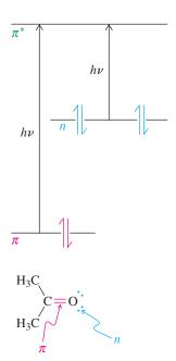
**Figure 17-6** The  $\pi \to \pi^*$  and  $n \to \pi^*$  transitions in acetone.
