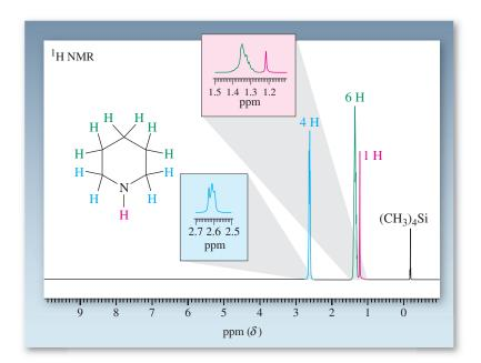
**Figure 21-4** 300-MHz <sup>1</sup>H NMR spectrum of azacyclohexane (piperidine). Like the OH hydrogen signal in alcohols, the amine NH peak may appear almost anywhere in the normal hydrogen chemical-shift range. Here the NH absorption occurs at  $\delta = 1.22$  ppm, and the signal is fairly sharp because of the use of dry solvent (CDCl<sub>3</sub>).
