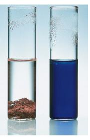
Addition of a molecule containing an aldehyde group to a solution of blue copper(II) sulfate (right) causes the formation of a brickred precipitate of copper(I) oxide in the Fehling test.
