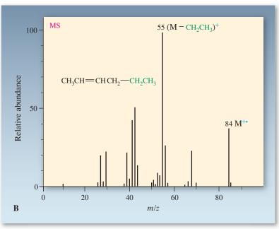
Branched and internal alkenes fragment similarly at allylic bonds. Figure 11-29B shows the mass spectrum of 2-hexene, in which the base peak at m/z = 55 corresponds to formation of the resonance-stabilized 2-butenyl cation.
