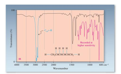
**Figure 11-19** IR spectrum of hexane. Comparison with that of pentane (Figure 11-18) shows that the location and appearance of the major bands are very similar, but the two fingerprint regions show significant differences at higher recorder sensitivity (in red).
