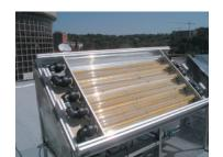
Photochemical reactions are used increasingly in "green" technology. This reactor on the roof of Complutense University of Madrid is used for water disinfection. A polymer-supported dye absorbs sunlight to convert oxygen to a more reactive state ("singlet oxygen"), which destroys harmful bacteria in water (picture courtesy of Professor Guillermo Orellana, UCM).
