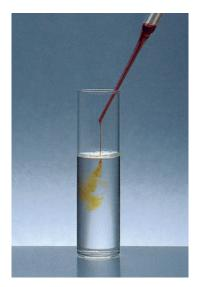
Addition of bromine to an alkene results in almost immediate loss of the red-brown color of Br<sub>2</sub> as the reaction takes place.
