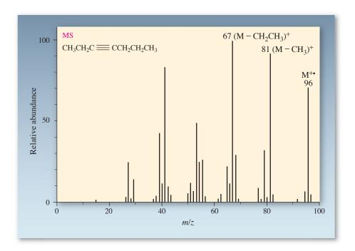
**Figure 13-7** Mass spectrum of 3-heptyne, showing M<sup>++</sup> at m/z = 96 and important fragments at m/z = 67 and 81 arising from cleavage of the C1–C2 and C5–C6 bonds.
