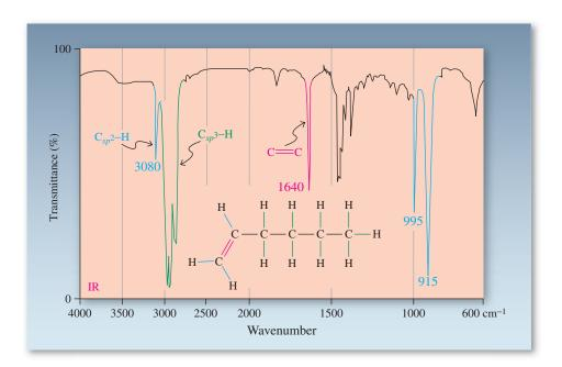
**Figure 11-20** IR spectrum of 1-hexene:  $\widetilde{\nu}_{\text{Csp}^2-\text{H stretch}} = 3080 \text{ cm}^{-1};$   $\widetilde{\nu}_{\text{C=C stretch}} = 1640 \text{ cm}^{-1};$   $\widetilde{\nu}_{\text{Csp}^2-\text{H bend}} = 995 \text{ and } 915 \text{ cm}^{-1}.$
