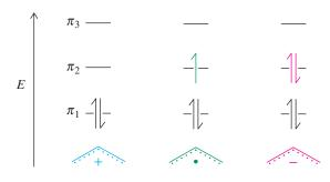
**Figure 14-3** The Aufbau principle is used to fill up the  $\pi$  molecular orbitals of 2-propenyl (allyl) cation, radical, and anion. In each case, the total energy of the  $\pi$  electrons is lower than that of three noninteracting p orbitals. Partial cation, radical, or anion character is present at the end carbons in these systems, a result of the location of the lobes in the  $\pi_2$  molecular orbital.
