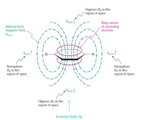
**Figure 15-9** The  $\pi$  electrons of benzene may be compared to those in a loop of conducting metal. Exposure of this loop of electrons to an external magnetic field  $H_0$  causes them to circulate. This "ring current" generates a local field, reinforcing  $H_0$  on the outside of the ring. Thus, the hydrogens resonate at lower field.
