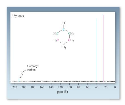
**Figure 17-4** <sup>13</sup>C NMR spectrum of cyclohexanone. The carbonyl carbon at 211.8 ppm is strongly deshielded relative to the other carbons. Because of symmetry, the molecule exhibits only four peaks; the three methylene carbon resonances absorb at increasingly lower field the closer they are to the carbonyl group.
