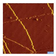
Scanning tunneling microscope (STM) image of a catalytic Pt surface. STM provides pictures at atomic resolution (the bar at the bottom right indicates 5 nm = 50 Å). You can see the highly ordered patterns of parallel arrays of Pt atoms in brown. The yellow "crosslines" indicate steps on the surface, on which much of the catalytic activity takes place. (Courtesy Professor Gabor A. Somorjai and Dr. Feng Tao, University of California at Berkeley.)
