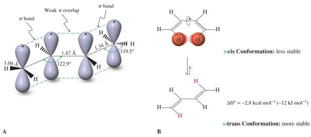
**Figure 14-6** (A) The structure of 1,3-butadiene. The central bond is shorter than that in an alkane (1.54 Å for the central C–C bond in butane). The *p* orbitals aligned perpendicularly to the molecular plane form a contiguous interacting array. (B) 1,3-Butadiene can exist in two planar conformations. The s-cis form shows steric hindrance because of the proximity of the two "inside" hydrogens highlighted in red.
