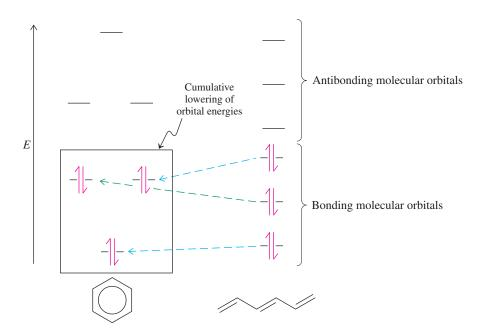
**Figure 15-5** Energy levels of the  $\pi$  molecular orbitals in benzene and 1,3,5-hexatriene. In both, the six  $\pi$  electrons fill the three bonding molecular orbitals. In benzene, two of them are lower in energy and one is higher than the corresponding orbitals in 1,3,5-hexatriene. Overall, energy is reduced and stability increased in going from the acyclic to the cyclic system.
