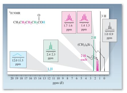
**Figure 19-2** 300-MHz <sup>1</sup>H NMR spectrum of pentanoic acid. The scale has been expanded to 20 ppm to allow the signal for the acid proton at  $\delta = 11.75$  ppm to be shown. The methylene hydrogens at C2 absorb at the next lowest field as a triplet ( $\delta = 2.35$  ppm, J = 7 Hz), followed by a quintet and a sextet, respectively, for the next two sets of methylenes. The methyl group appears as a distorted triplet at highest field ( $\delta = 0.92$  ppm, J = 6 Hz).
