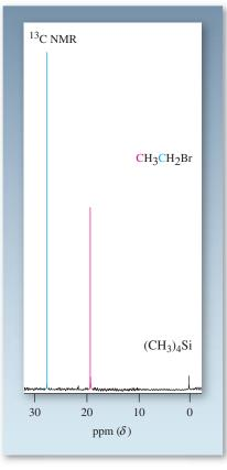
**Figure 10-31** This 62.8-MHz <sup>13</sup>C NMR spectrum of bromoethane was recorded with broad-band decoupling at 250 MHz. All lines simplify to singlets, including the absorption for (CH<sub>3</sub>)<sub>4</sub>Si.
