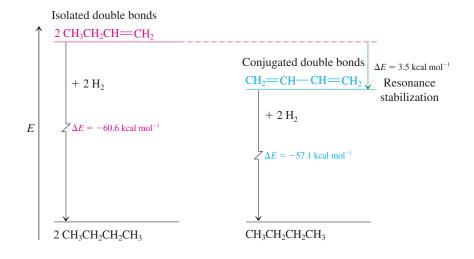
**Figure 14-5** The difference between the heats of hydrogenation of two molecules of 1-butene (a terminal monoalkene) and one molecule of 1,3-butadiene (a doubly terminal conjugated diene) reveals their relative stabilities. The value, about 3.5 kcal mol<sup>-1</sup>, is a measure of the stabilization of 1,3-butadiene due to conjugation.
