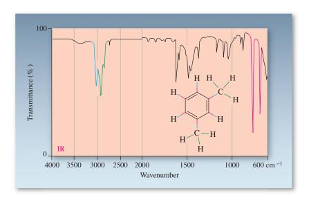
**Figure 15-7** The infrared spectrum of 1,3-dimethylbenzene (*m*-xylene). There are two C-H stretching absorptions, one due to the aromatic bonds (3030 cm<sup>-1</sup>), the other to saturated C-H bonds (2920 cm<sup>-1</sup>). The two bands at 690 and 765 cm<sup>-1</sup> are typical of 1,3-disubstituted benzenes.
