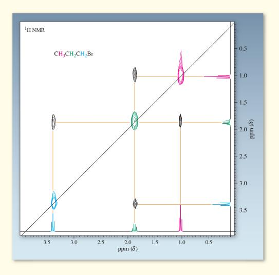
The two spectra along the x and y axes are identical to that in Figure 10-27. The marks on the diagonal line correlate the same peaks in each spectrum (indicated by the colored "blotches") and can be ignored. It is the off-diagonal correlations (indicated by the orange lines) that prove the connectivity of the hydrogens in the molecule. Thus, the (red) methyl triplet at  $\delta=1.05$  ppm has a cross peak (indicated
