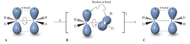
**Figure 11-6** Thermal isomerization of *cis*-dideuterioethene to the trans isomer requires breaking the  $\pi$  bond. The reaction proceeds from starting material (A) through rotation around the C–C bond until it reaches the point of highest energy, the transition state (B). At this stage, the two p orbitals used to construct the  $\pi$  bond are perpendicular to each other. Further rotation in the same direction results in a product in which the two deuterium atoms are trans (C).
