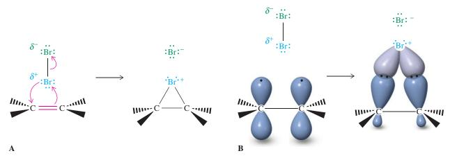
**Figure 12-3** (A) Electron-pushing picture of cyclic bromonium ion formation. The alkene (red) acts as a nucleophile to displace bromide ion (green) from bromine. The molecular bromine behaves as if it were strongly polarized, one atom as a bromine cation, the other as an anion. (B) Orbital picture of bromonium ion formation.
