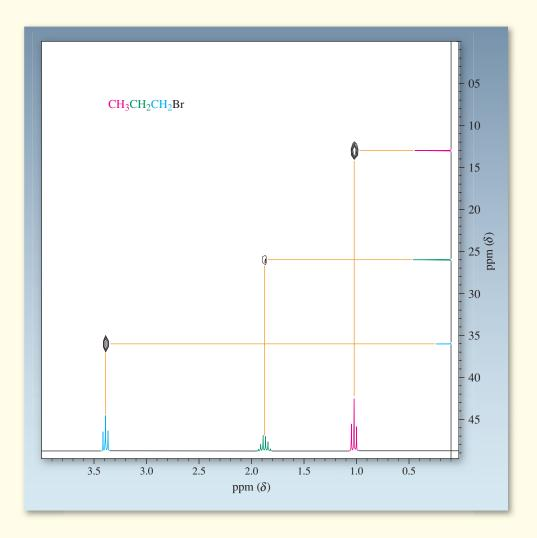
The  $^{13}$ C NMR spectrum is plotted on the *y* axis and exhibits three peaks. On the basis of what we know about carbon NMR, we can readily assign the signal at  $\delta=13.0$  ppm to the methyl carbon, that at  $\delta=26.2$  ppm to the methylene, and that at  $\delta=36.0$  ppm to the bromine-bearing carbon. But even without this knowledge, these assignments are immediately evident from the cross-correlations of the
