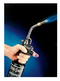
Propane stored under pressure in liquefied form in canisters such as these is a common fuel for torches, lanterns, and outdoor cooking stoves. [Courtesy Bernzomtic, Columbus, OH.]
