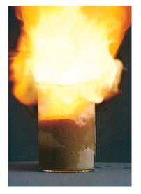
Vivid demonstration of the combustion of ethyne, generated by the addition of water to calcium carbide.
