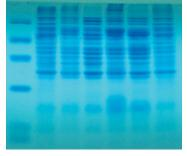
Electrophoresis of proteins on polyacrylamide. Each column of blue bands illustrates the separation of a mixture of proteins into their individual components.
