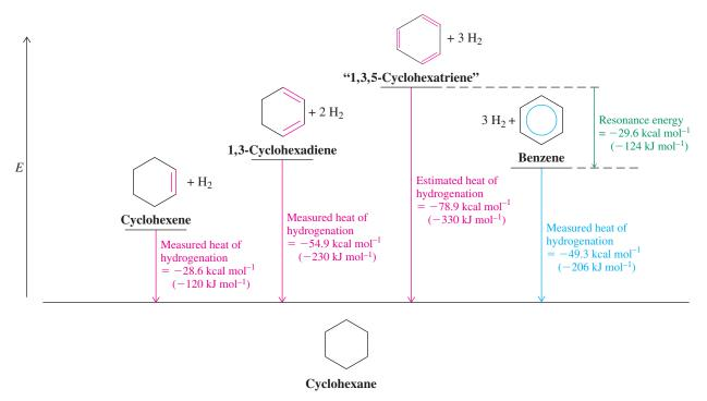
**Figure 15-3** Heats of hydrogenation provide a measure of benzene's unusual stability. Experimental values for cyclohexene and 1,3-cyclohexadiene allow us to estimate the heat of hydrogenation for the hypothetical "1,3,5-cyclohexatriene." Comparison with the experimental  $\Delta H^{\circ}$  for benzene gives a value of approximately 29.6 kcal mol<sup>-1</sup> for the aromatic resonance energy.
