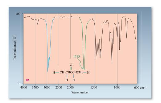
**Figure 17-5** IR spectrum of 3-pentanone;  $\tilde{v}_{C=O \text{ stretch}} = 1715 \text{ cm}^{-1}$ .
