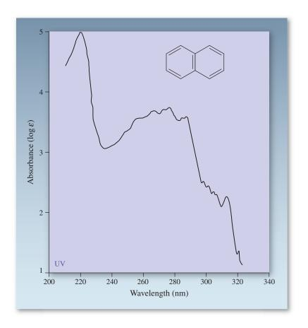
**Figure 15-13** Extended  $\pi$  conjugation in naphthalene is manifest in its UV spectrum (measured in 95% ethanol). The complexity and location of the absorptions are typical of extended  $\pi$  systems.
