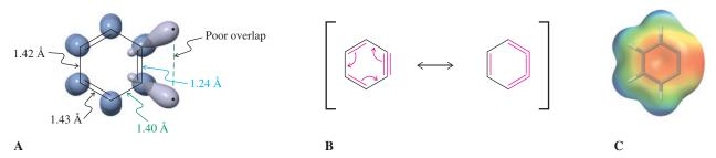
**Figure 22-4** (A) The orbital picture of benzyne reveals that the six aromatic  $\pi$  electrons are located in orbitals that are perpendicular to the two additional hybrid orbitals making up the distorted triple bond. These hybrid orbitals overlap only poorly; therefore, benzyne is highly reactive. (B) Resonance in benzyne. (C) The electrostatic potential map of benzyne shows electron density (red) in the plane of the six-membered ring at the position of the distorted sp-hybridized carbons.
