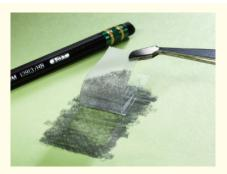
How to obtain a Nobel Prize: peeling off graphene from graphite using Scotch tape.
