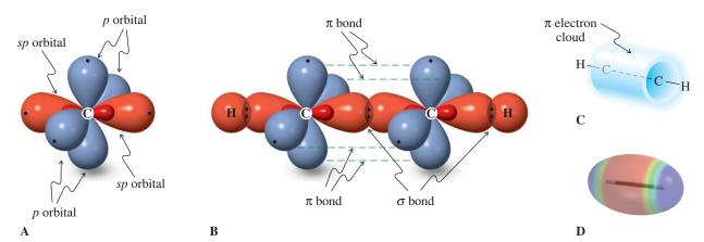
**Figure 13-1** (A) Orbital picture of *sp*-hybridized carbon, showing the two perpendicular p orbitals. (B) The triple bond in ethyne: The orbitals of two *sp*-hybridized CH fragments overlap to create a  $\sigma$  bond and two  $\pi$  bonds. (C) The two  $\pi$  bonds produce a cylindrical electron cloud around the molecular axis of ethyne. (D) The electrostatic potential map reveals the (red) belt of high electron density around the central part of the molecular axis.
