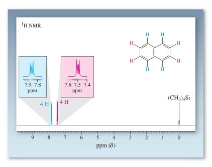
**Figure 15-16** The 300-MHz  $^1$ H NMR spectrum of naphthalene reveals the characteristic deshielding due to a  $\pi$ -electronic ring current.
