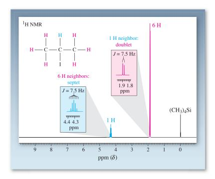
**Figure 10-22** 300-MHz <sup>1</sup>H NMR spectrum of 2-iodopropane:  $\delta = 4.31$  (sep, J = 7.5 Hz, 1 H), 1.88 (d, J = 7.5 Hz, 6 H) ppm. The six equivalent nuclei on the two methyl groups give rise to a septet for the tertiary hydrogen (N + 1 rule).
