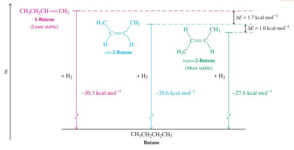
**Figure 11-12** The relative energy contents of the butene isomers, as measured by their heats of hydrogenation, tell us their relative stabilities. The diagram is not drawn to scale.
