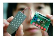
The world's smallest direct methanol fuel cell.
