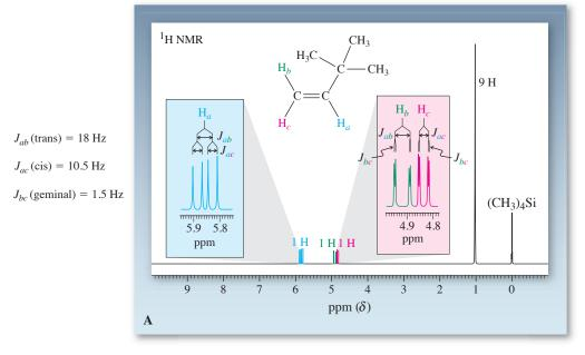
**Figure 11-11** 300-MHz <sup>1</sup>H NMR spectra of (A) 3,3-dimethyl-1-butene and (B) 1-pentene.
