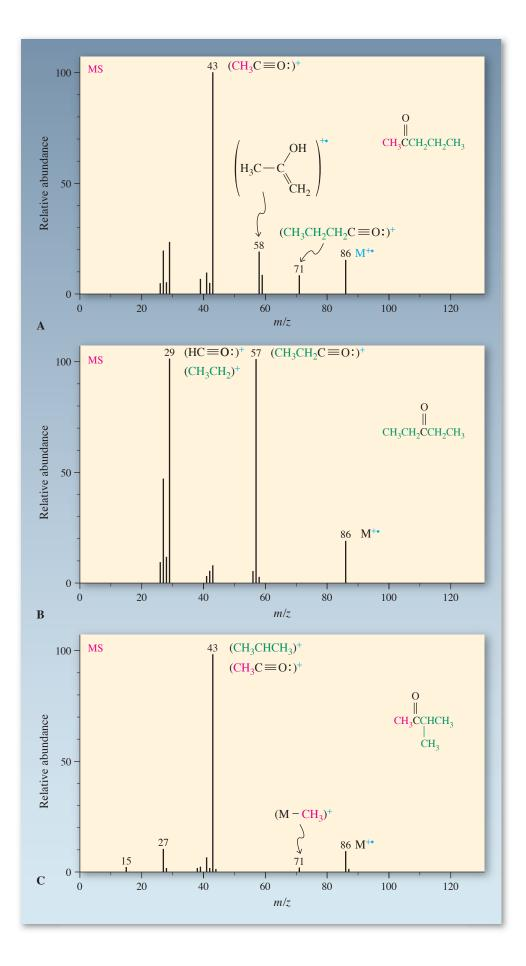
**Figure 17-7** Mass spectra of (A) 2-pentanone, showing two peaks for  $\alpha$  cleavage and one for McLafferty rearrangement; (B) 3-pentanone, showing only a single  $\alpha$  cleavage peak because of symmetry; and (C) 3-methyl-2-butanone, showing two  $\alpha$  cleavages.
