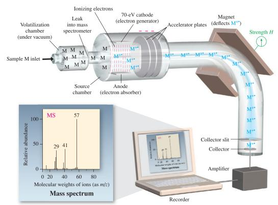
**Figure 11-22** Diagram of a mass spectrometer.
