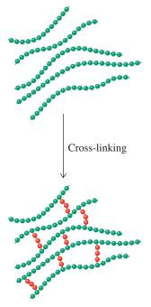
**Figure 14-12** Cross-linking underlies the elasticity of polybutadiene chains in rubber.
