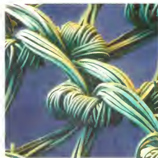
Scanning electron micrograph of the material in a nylon stocking. Sheer stockings require long, continuous fibers of small diameter and enormous strength. (Magnification 150X.)
