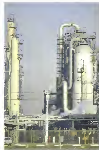
The large distillation tower at left is used to separate petroleum into fractions based on their boiling points. The “cat cracker” at right uses catalysts and high temperatures to crack large molecules into smaller ones.
