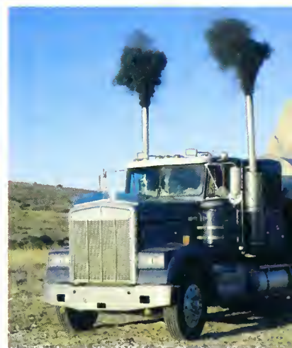
The black material in diesel exhaust consists of small particles that are rich in polynuclear aromatic hydrocarbons.
