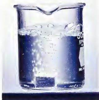
Sodium metal reacts vigorously with simple primary alcohols such as ethanol.
