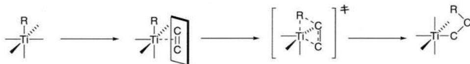
Scheme 1.27. Mechanism of coordination polymerization of olefins.
