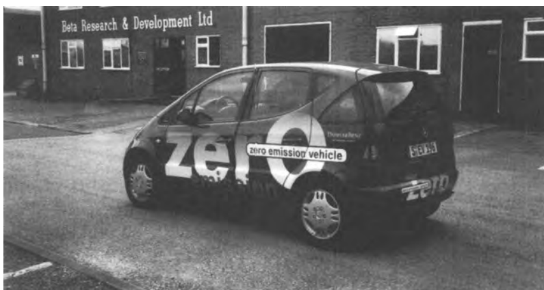
Figure 12.7 Electric version of Mercedes 'A class' car with sodium–nickel–chloride batteries
