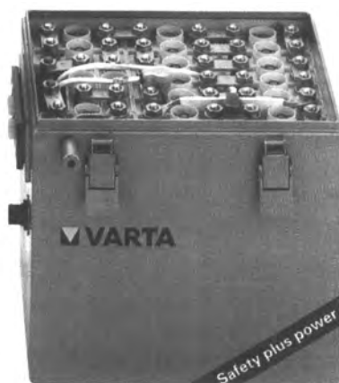
Figure 9.4 Nickel–cadmium aircraft battery (24 V) (By courtesy of Varta Batterie AG)
