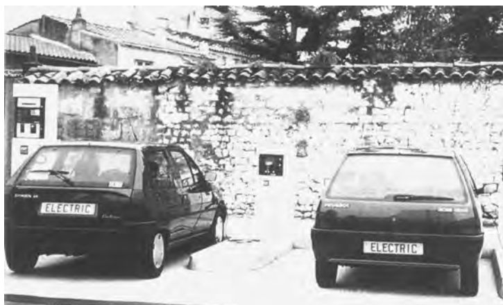
Figure 12.6 Electric versions of Citroën AX and Peugeot 106 cars with nickel–cadmium batteries (By courtesy of UK & International Press)
