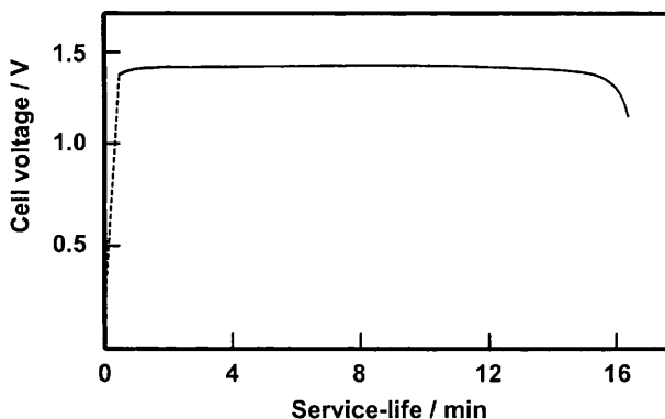
Figure 7.3 Discharge of high-rate zinc–silver-oxide cell at 20^\circ\text{C} (By courtesy of Research Studies Press Ltd.)
