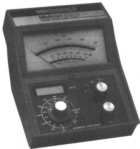
Figure 4.8 Simple battery-conductance test meters in (a) digital form and (b) analogue form (By courtesy of Batteries International)
