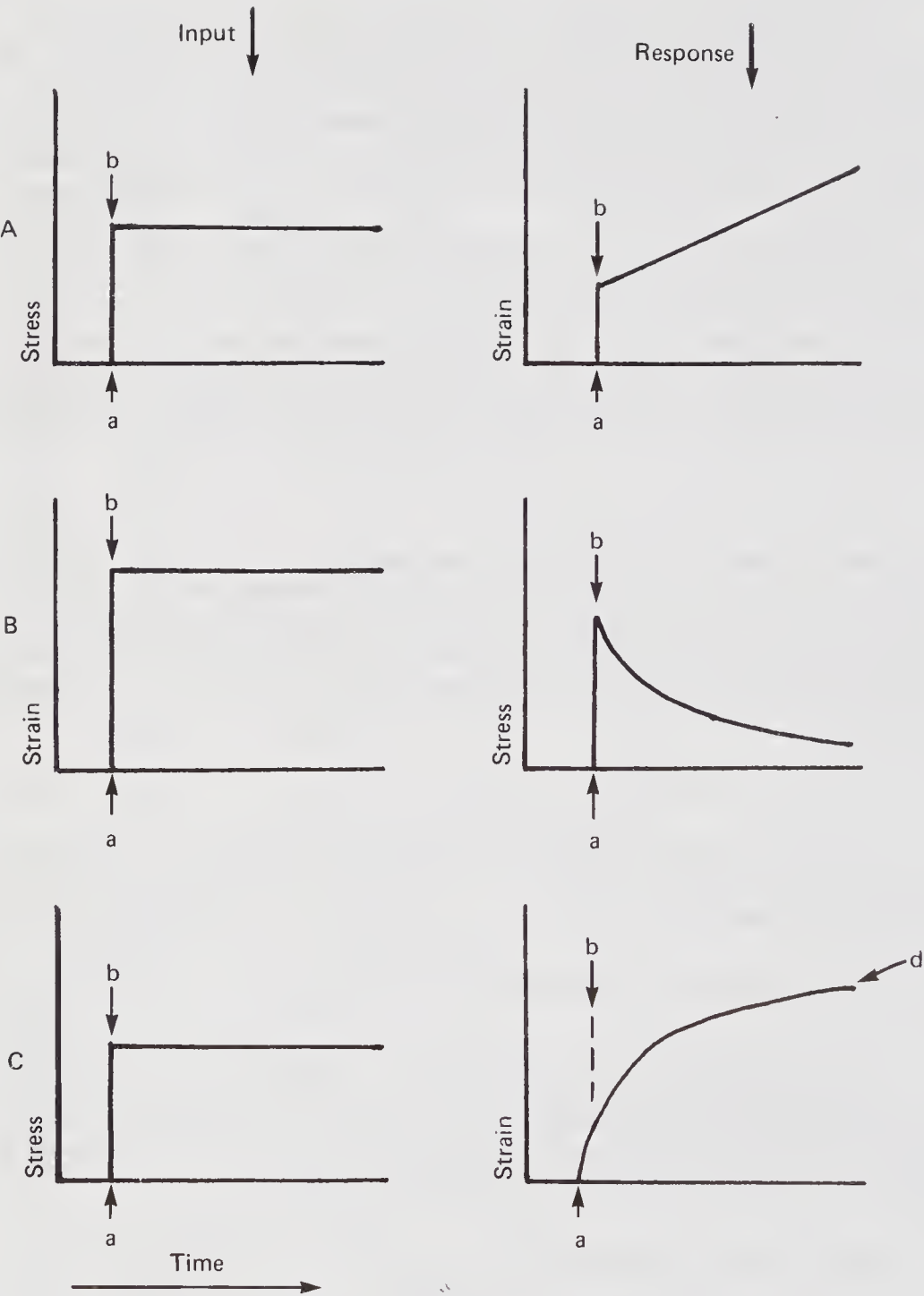
FIGURE 5.4 Stress-strain relationships for the Maxwell model (A and B) and the Voigt model (C).
