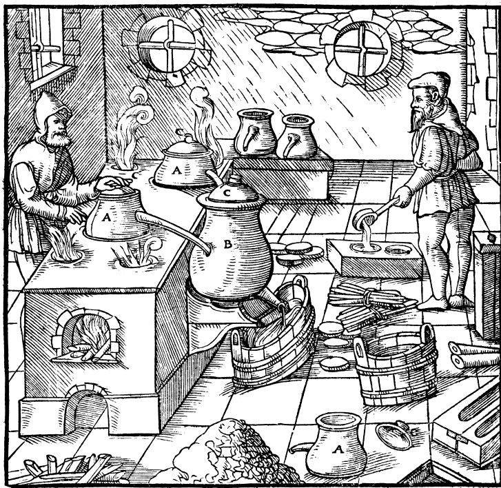
Fig. 27. A woodcut showing the distillation of sulfur from Agricola's De re metallica , 1556. The impure sulfur is heated in the pots (A) and the vapour from the boiling sulfur is fed into a larger pot (B), where it condenses to a liquid that drains out the spout at the bottom. The liquid may then be poured into moulds to form round cakes, or into wooden tubes moistened beforehand to make it easy to extract the rods of sulfur known as 'roll sulfur', shown in bundles on the floor.
