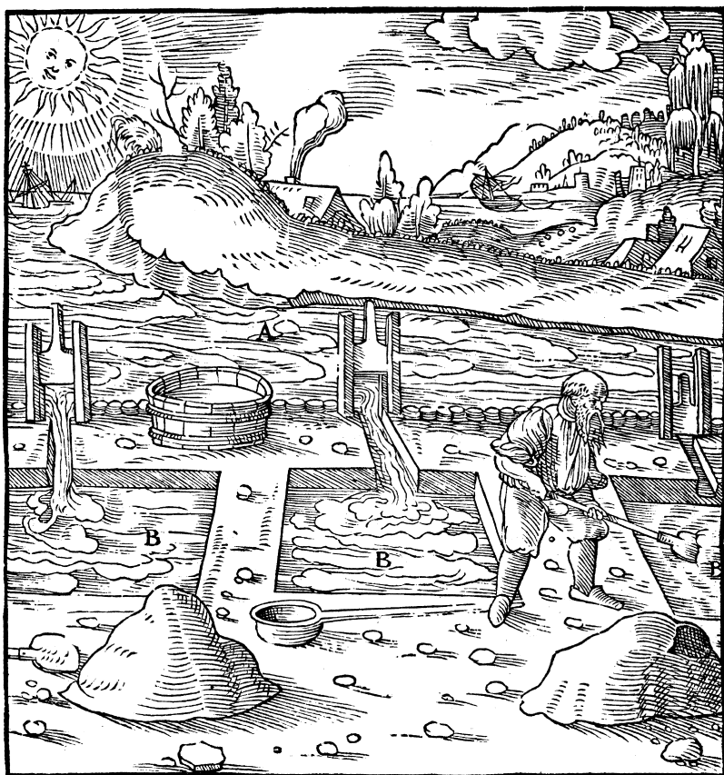
Fig. 34. A woodcut from the 1556 work De re metallica by Agricola. Water from the River Nile flows into the nitrum pits (B), from where the nitre crystals are collected after evaporation of the water.
