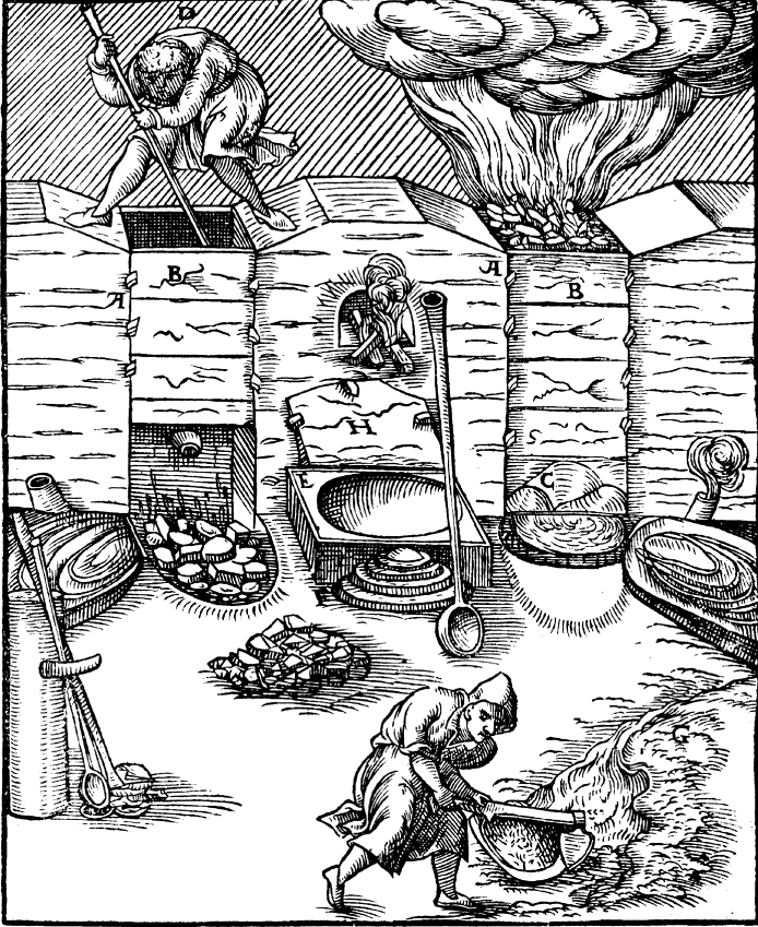
Fig. 25. Woodcut from Ercker (1580), showing the collection of cadmia or tutty by scraping the chimney of a furnace.
