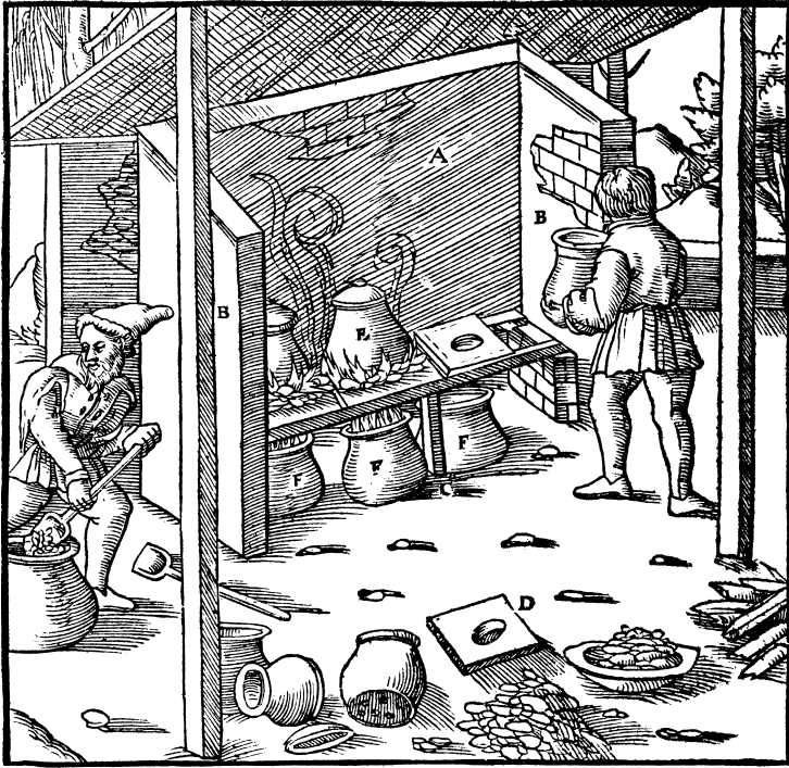
Fig. 28. A woodcut from Agricola's De re metallica from 1556 showing the production of sulfur from pyrites. The ore is packed into a vessel with holes in its base (E) and this is placed on an iron plate with a hole in it (D). After lighting a fire around the vessel, molten sulfur is liberated, and it falls into pots of water placed below (F).
