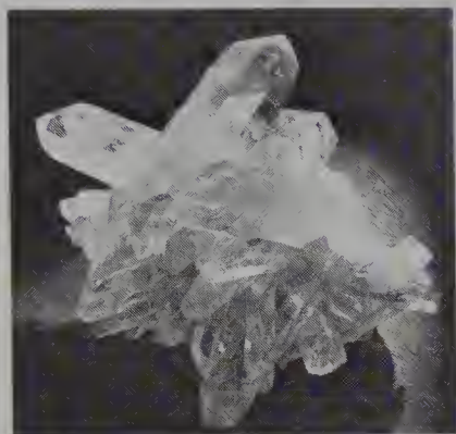
Fig. 2.9. Silicon dioxide. (a) Each Si atom (small spheres) is tetrahedrally bonded to four O atoms (large spheres), and each O atom is bonded to two Si atoms, forming a three-dimensional network that can be considered a giant molecule. There are three forms of \text{SiO}_2 , also called silica. (b) Crystals of quartz, one of the three forms of \text{SiO}_2 .
