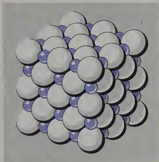
Fig. 1.3. Sodium chloride crystal. The larger spheres are the chloride ( \text{Cl}^- ) ions, and the smaller spheres are the sodium ( \text{Na}^+ ) ions.
