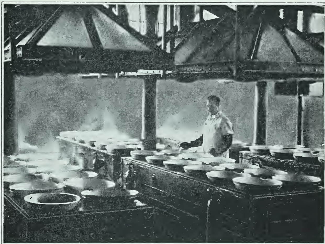
FIG. 37. Evaporating liquids in the manufacture of chemicals. What is the advantage of having the vessels of the shape shown in the figure?
