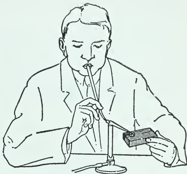
FIG. 328. Heating a metal in the oxidizing flame
