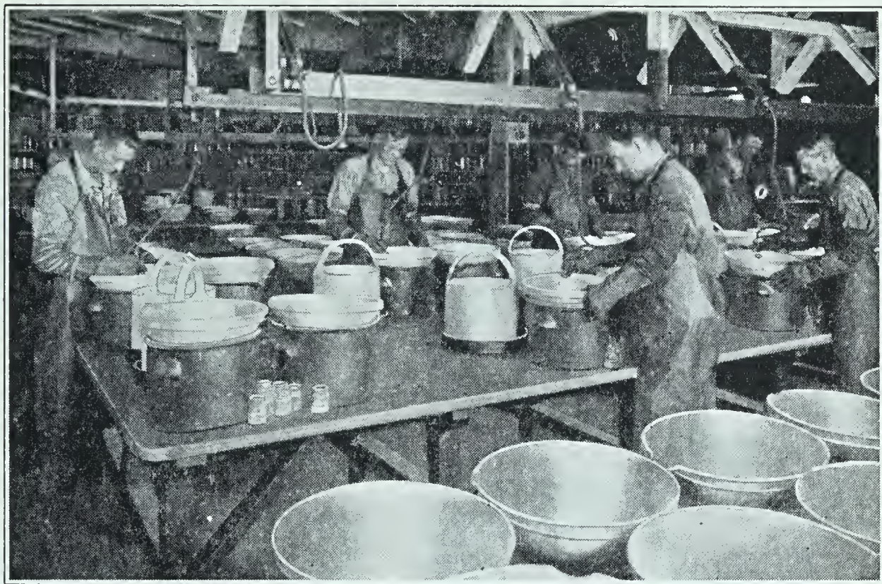
FIG. 215. Preparing silver nitrate by dissolving silver in nitric acid. Large quantities of the nitrate are used in preparing compounds needed in photography
