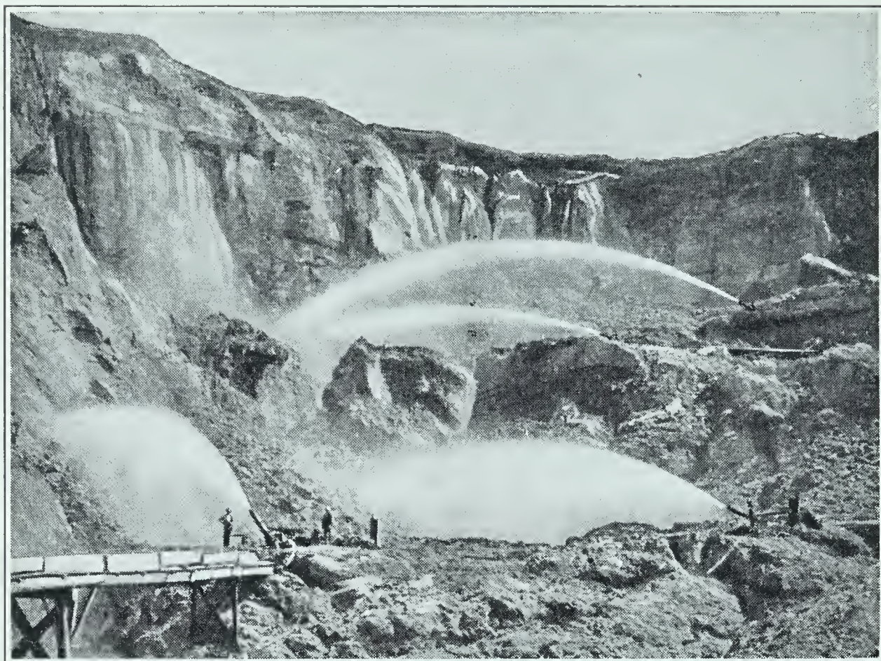
FIG. 456. The hydraulic mining of gold. The gold-bearing rocks are broken down by powerful streams of water
