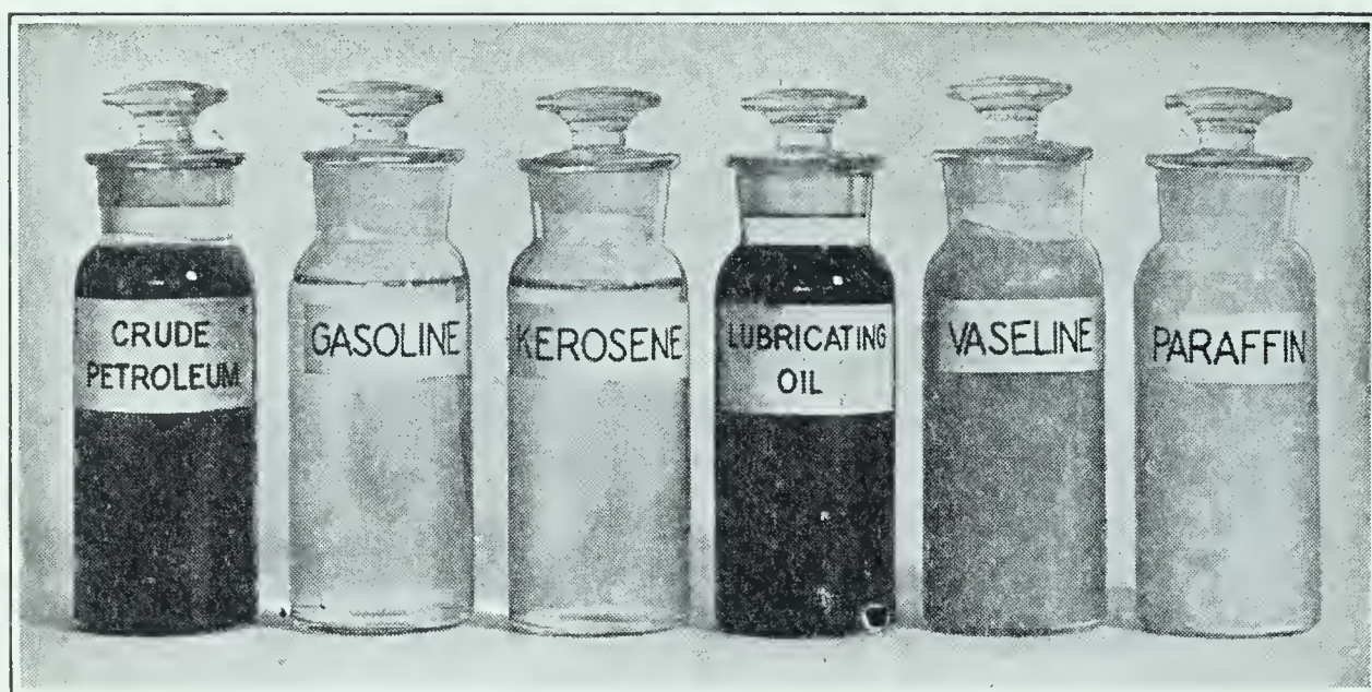
FIG. 313. Crude petroleum and some important products obtained from it
