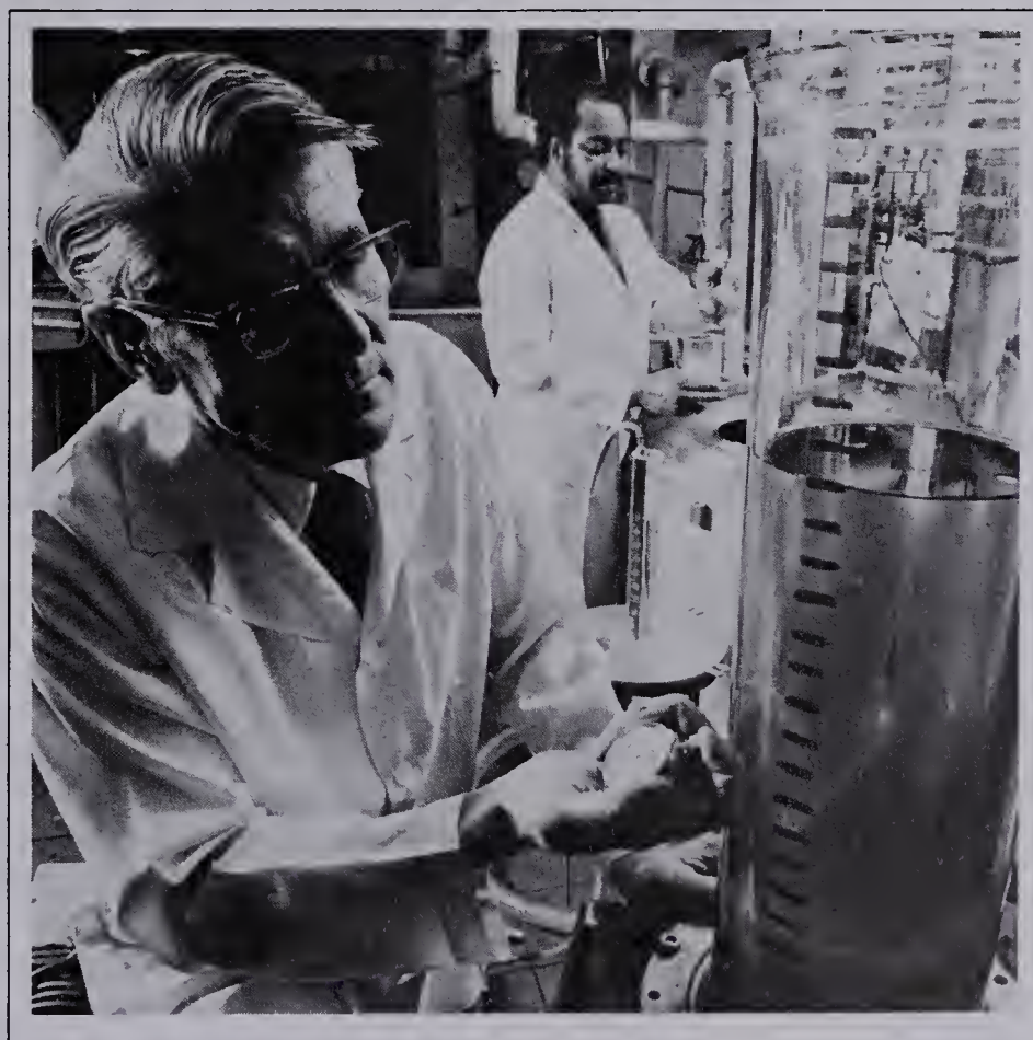
Biochemists measure the flow rate of milk through a homogenizer. (U.S. Dept. of Agriculture photo by Jim Strawser.)
