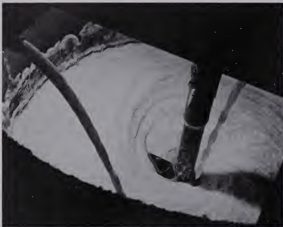
Soap is formed in this neutralizer tank when a stream of fatty acids is mixed with a stream of alkali. (Courtesy of Proctor and Gamble Company.)
