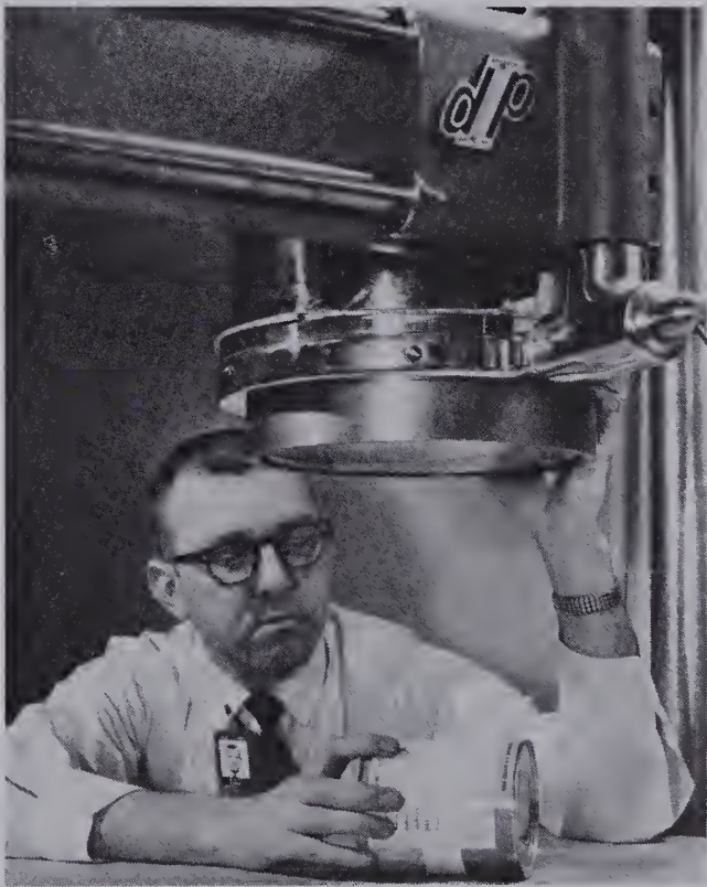
A sample can of paint being placed under a gamma scintillation counter at Oak Ridge, Tennessee. Radiation from the sample will then be counted to determine its radioactivity content. The scientist is wearing a radiation badge on his shirt. (Photo courtesy of Union Carbide Corp.)
