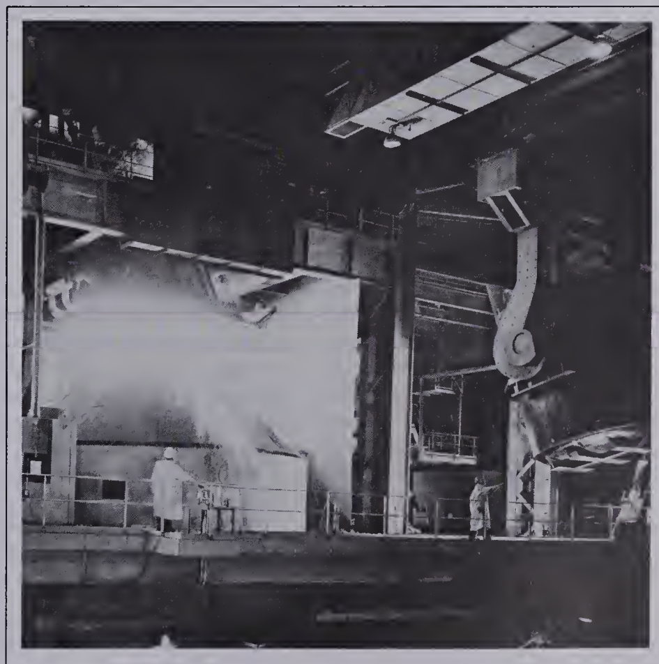
Basic oxygen furnace in operation. (Courtesy of the American Iron and Steel Institute.)
