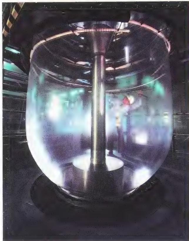
Polyethylene film, which is widely used for packaging, is formed by extruding the molten plastic through a ringlike gap and inflating it like a balloon
