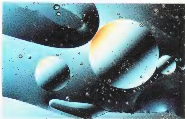
A polarized light view of light heating oil. The colors arise from the interference of rays that take different times to pass through the liquid and show regions of different density and molecular packing.
