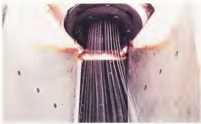
In the industrial version of a spider's spinneret (see pages 93–94), nylon is being extruded as thread.
