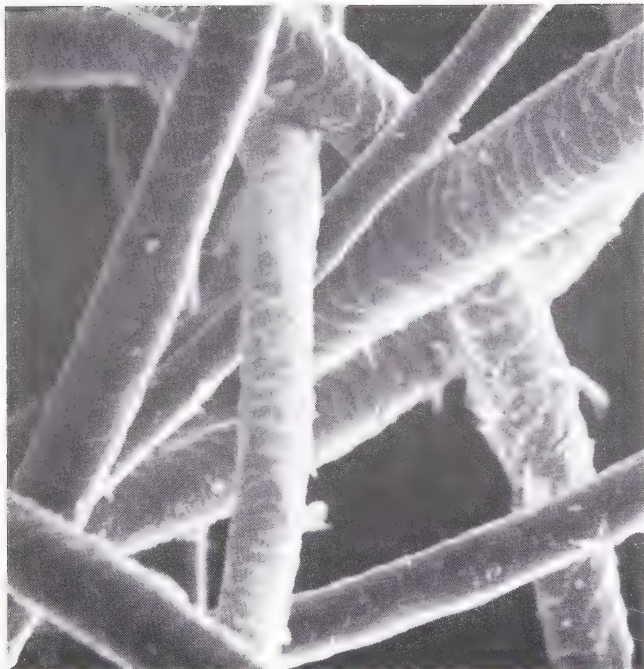
Wool fibers. The scales are responsible for the formation of felt, for they lock the fibers into a dense tangle when they are rubbed together.
