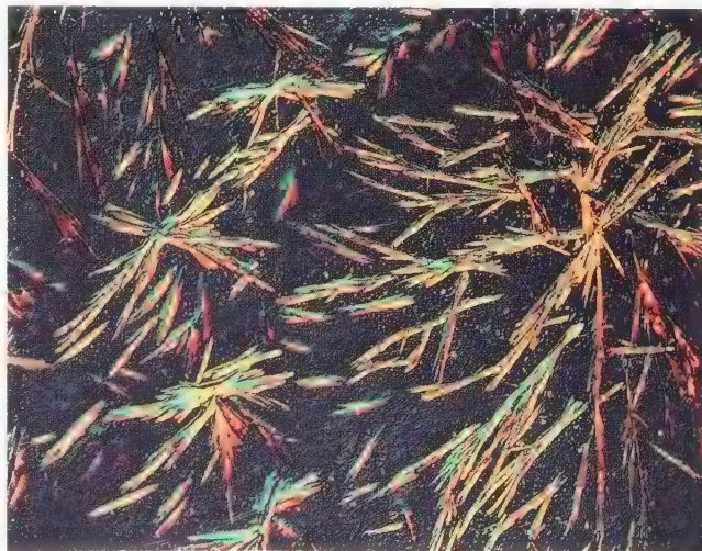
Left- and right-handed molecules of lactic acid exist and crystallize into colonies of the same type. The presence of the two types is shown by different colors when a sample is examined with a polarizing microscope.
