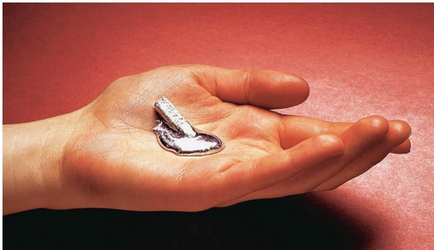
Of all the elements, gallium has the largest temperature range over which it is in the liquid state at atmospheric pressure. (Charles D. Winters/Photo Researchers)
