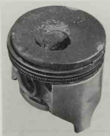
A piston head damaged by severe knocking.
