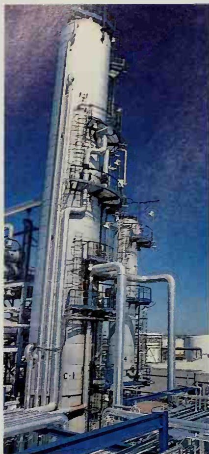
A fractionating tower. Distillation of crude oil in towers like this separates the hydrocarbons of the petroleum into fractions useful as gasoline, kerosene, heating oil, jet fuel, and so on.
