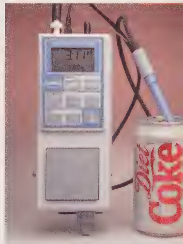
Figure 10.6 A pH meter, an instrument used for the very accurate measurement of hydrogen ion concentrations.
