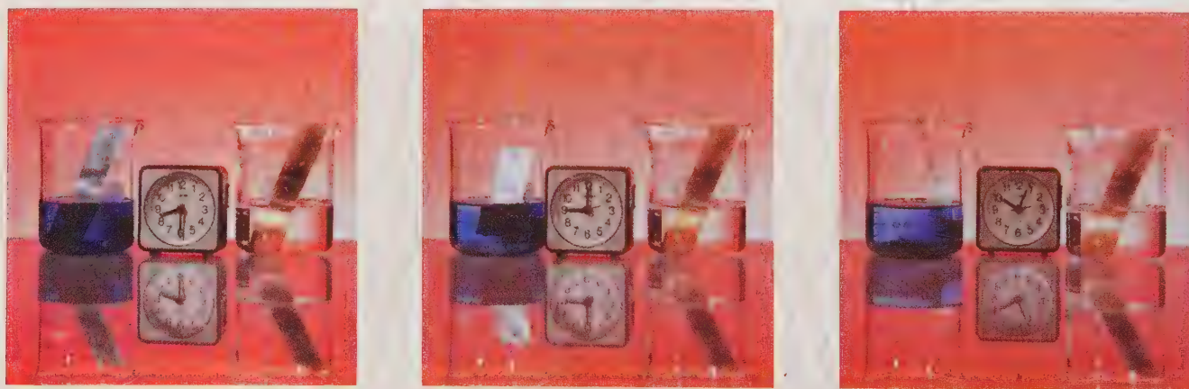
Figure 11.5 Zinc metal and copper sulfate. As time passes, the zinc strip erodes, dark granules of copper appear, and the blue color of the copper solution fades. Zinc atoms of the metal strip are oxidized to colorless zinc ions as blue copper ions in the solution are reduced to copper atoms. Meanwhile, copper metal accumulates at the bottom of the beaker. No change occurs in the beaker holding the copper strip immersed in a solution of zinc sulfate.
