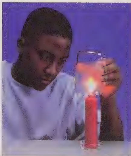
Figure 6.1 Observing the chemistry of a burning candle. As you lower a beaker over a candle flame, you first see evidence of the water that is formed on combustion of the hydrocarbons. Then, as the oxygen in the beaker is replaced by carbon dioxide, the flame dies.
