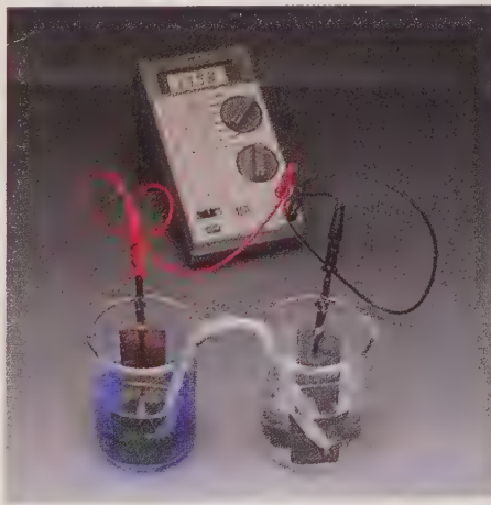
Figure 11.4 A form of the Daniell cell. The sodium chloride of the salt bridge acts as an electrolyte and allows ions to flow between the two beakers, generating almost 1.1 volts.
