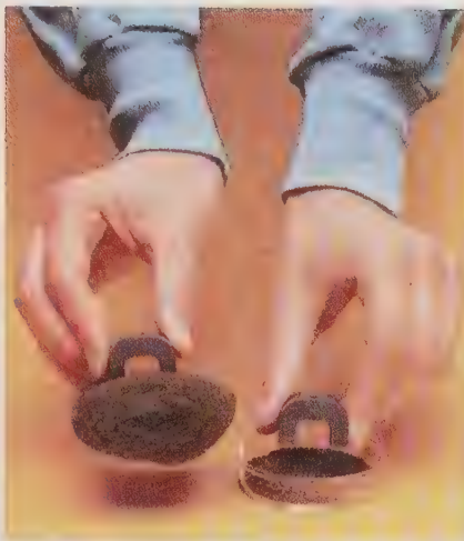
Figure 3.1 The attraction that iron has for a magnet isn't carried over into the iron oxides it forms as it rusts.
