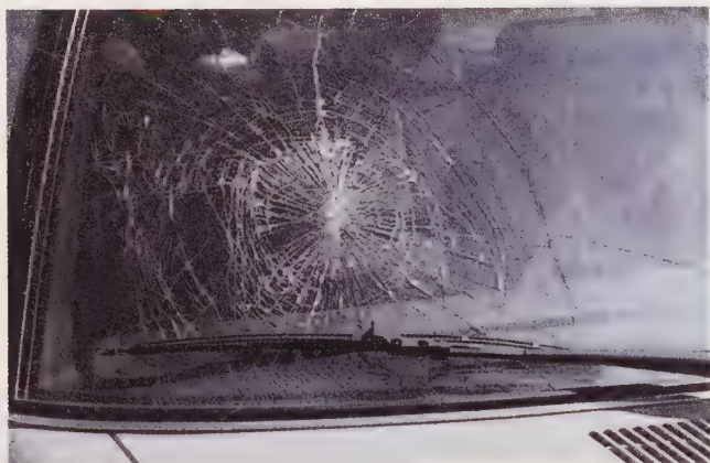
A broken car window made of safety glass. A sheet of polyvinylacetate sandwiched between two sheets of glass prevents the broken glass from disintegrating into flying slivers.
