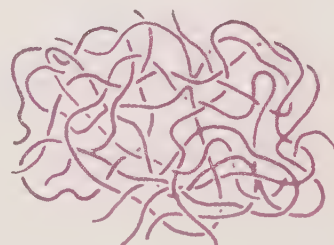
Figure 21.20 Disorganized polymeric strands of low-density polyethylene.
