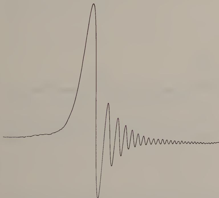
Figure 7. Ringing (or "wiggles") seen after passage through resonance. Direction of scan is from left to right.
