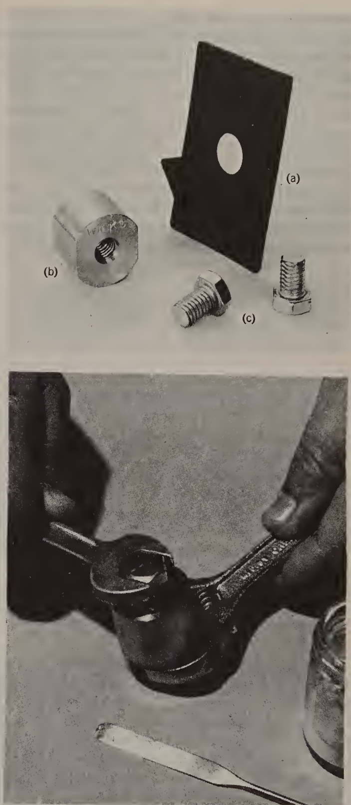
Figure 6. Mini-press and operation. (a) Cell holder. (b) Nut = cell. (c) Bolts.
