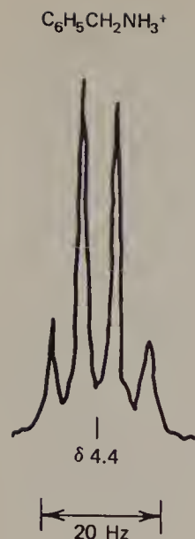
Figure 31. NMR spectrum of \alpha methylene unit of a primary amine in \text{CF}_3\text{CO}_2\text{H} ; corresponds to Table II, first line.
