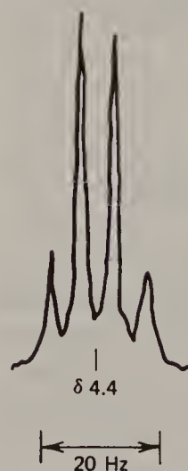
FIGURE 4.35. NMR spectrum of \alpha -methylene unit of a primary amine at 100 MHz in \text{CF}_3\text{CO}_2\text{H} ; corresponds to Table 4.1, first line.
