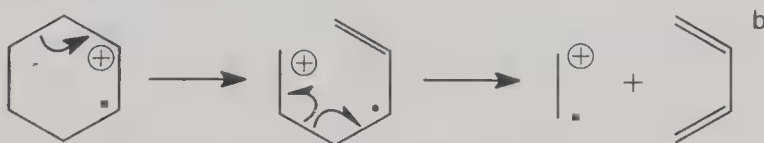
Figure 6.15. The retro Diels–Alder fragmentation can proceed either by charge retention or charge migration. (a) Charge-retention (charge retained by the diene fragment); (b) charge-migration (charge transferred to olefin fragment). Many substituents are possible.
