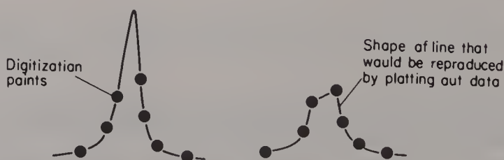
Fig. 5.10 Effect of digitization on a Lorentzian NMR signal.
