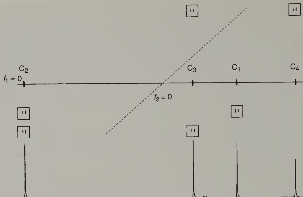
Fig. 4.27. ^{13}\text{C} INADEQUATE spectrum of 2-butanol, 4.1. The sample was neat butanol containing 20% acetone- \text{d}_6 that was added to provide a lock.
