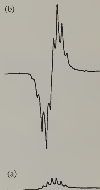
Fig. 3.39. The 79.5 MHz natural abundance ^{29}\text{Si} spectrum of \text{Me}_3\text{SiCl} , (a) without polarization transfer or NOE, and (b) using INEPT.
