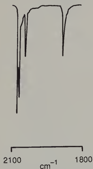
Fig. 7.6. Room-temperature IR spectrum of \text{Rh}_4(\text{CO})_{12} , 7.3, in cyclohexane solution, demonstrating slow exchange.
