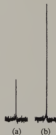
Fig. 6.8. ^{13}\text{C} signal of C_2 of 2-butanol, (a) without, and (b) with, ^1\text{H} NOE. In each case a single transient was acquired proton-decoupled.
