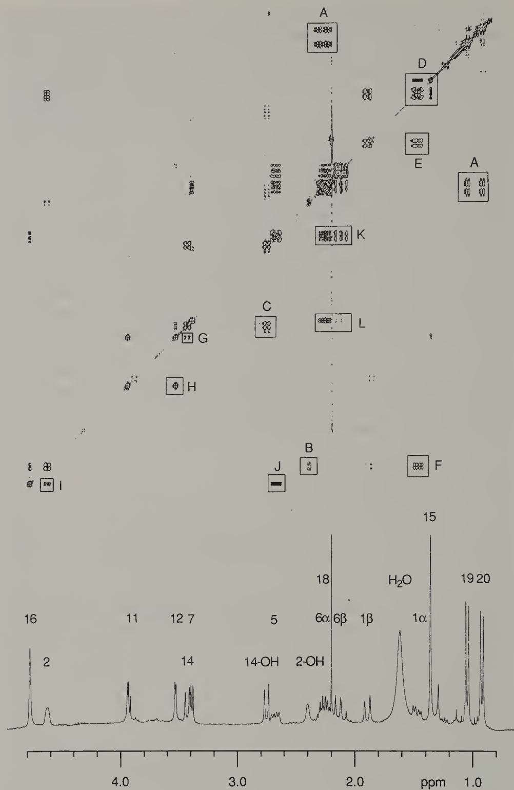
Fig. 5.3. 300 MHz DQF-PS COSY spectrum of tripdiolide, 5.14 , c. 1 mM in CDCl 3 solution. For clarity, the spectrum is plotted in a single colour. 512 increments were acquired, with 64 transients acquired for each; the spectral window was \pm 660 Hz in each dimension; the final size of the spectrum after zero filling was 2K in f_2 (giving 0.65 Hz/point) \times 1K in f_1 (giving 1.3 Hz/point).
