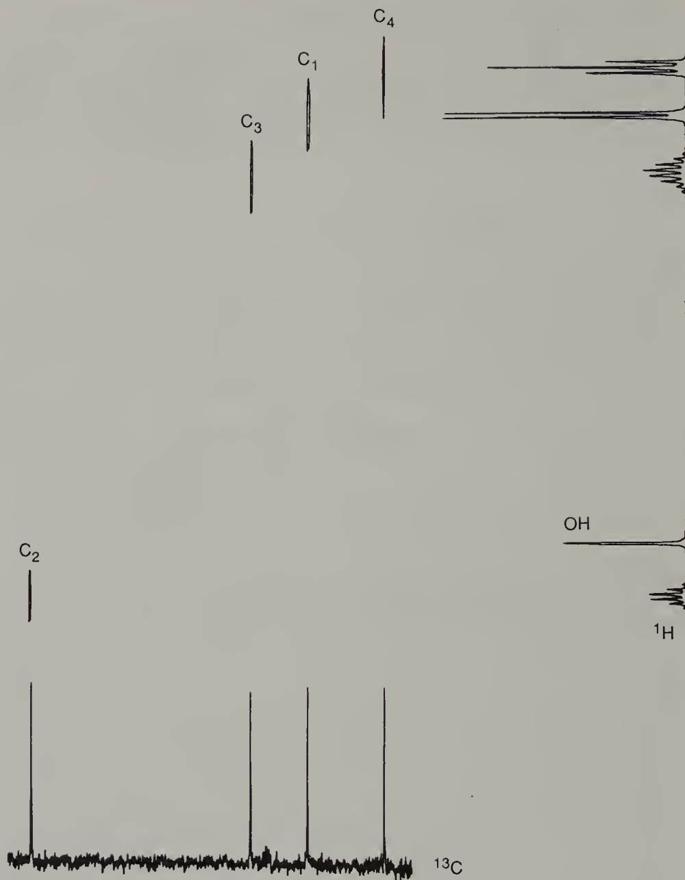
Fig. 4.8. Two-dimensional 62.9 MHz ^1\text{H} - ^{13}\text{C} chemical shift correlation spectrum of 2-butanol, 4.1. Also shown are the corresponding one-dimensional ^1\text{H} and ^{13}\text{C} spectra.
