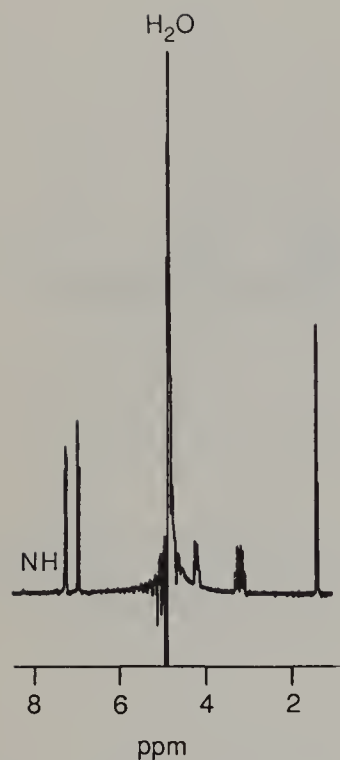
Fig. 8.12. The same sample as Fig. 8.11, subjected to presaturation of the water signal.
