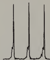
Fig. 7.11. ^1\text{H} spectrum of \text{NH}_4^+ in acidified \text{H}_2\text{O}/\text{D}_2\text{O} . J(^{14}\text{N}-^1\text{H}) \approx 52 Hz. The additional signals on the low-field edge of each line are due to small amounts of isotopically shifted \text{NH}_3\text{D}^+ .
