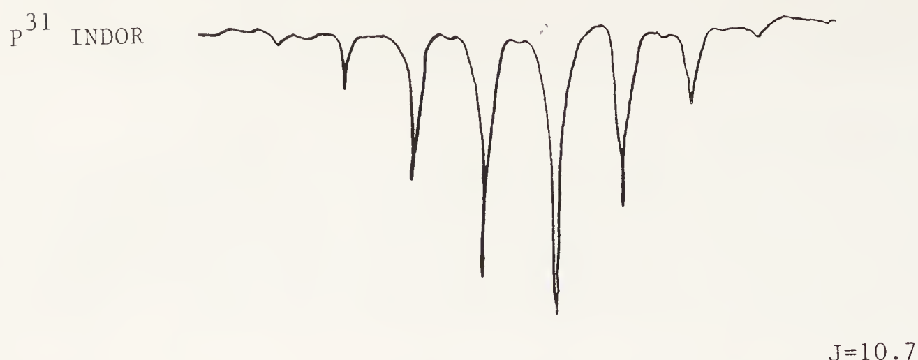
Figure 9.15. INDOR spectrum of (\text{CH}_3\text{O})_3\text{P} . [From E. B. Baker, L. W. Burd, and C. V. Root, Rev. Sci. Instrum. 34 , 243 (1963).]
