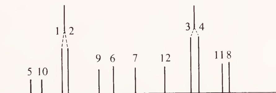
Figure 7.13. Portion of an A_2B_2 spectrum with J_{AB} much larger than J'_{AB} .
