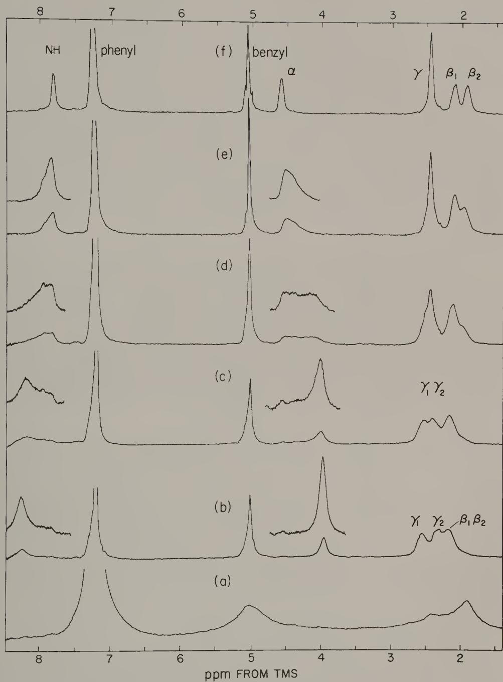
Fig. 7.16. 300 MHz spectra of poly- \gamma -benzyl L -glutamate of \overline{DP} \sim 160 in \text{CDCl}_3 (5% wt./vol.) at 32^\circ\text{C} . The volume percent of trifluoroacetic acid added is (a) 0%; (b) 10%; (c) 12%; (d) 13%; (e) 16%, (f) 20%. [F. A. Bovey and F. C. Schilling, Macromol. Rev. 9 , 1 (1975).]
