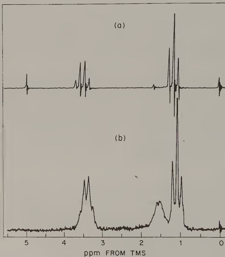
Fig. 7.1. 60 MHz proton spectra of (a) ethyl orthoformate \text{HC}(\text{OCH}_2\text{CH}_3)_3 and (b) poly(vinyl ethyl ether), both observed in 15% (wt./vol.) solution in carbon tetrachloride at ca. 25°C. (A. I. R. Brewster, private communication.)
