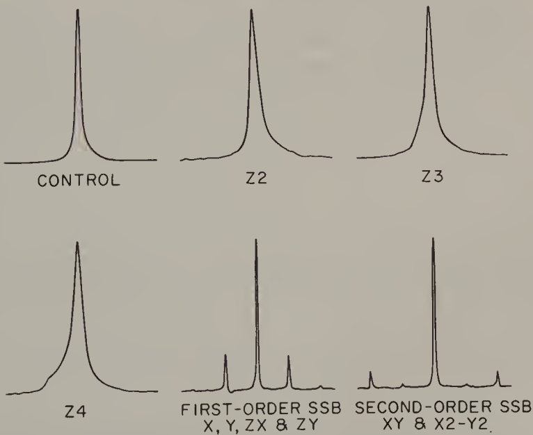
Fig. 2.6. Deliberate misadjustment of various shims for a superconducting magnet. (Adapted from Ref. 5.)
