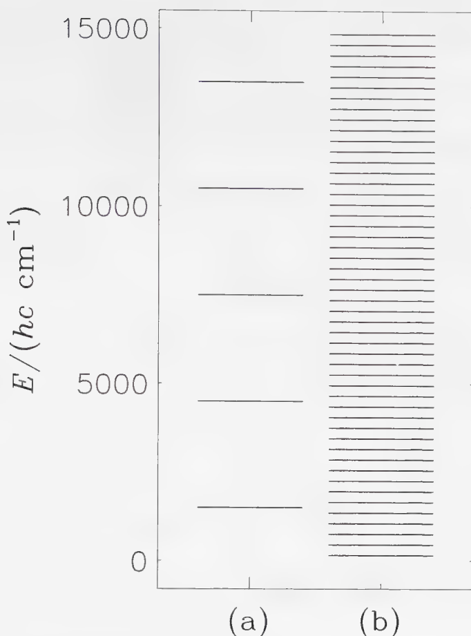
Figure 4.2. The term values for two different harmonic-oscillator potentials: In (a) the force constant \lambda is 3.19 \times 10^{29} \text{ s}^{-2} ( \omega_e = 3000 \text{ cm}^{-1} ), and in (b) \lambda = 3.19 \times 10^{27} \text{ s}^{-2} ( \omega_e = 300 \text{ cm}^{-1} ).
