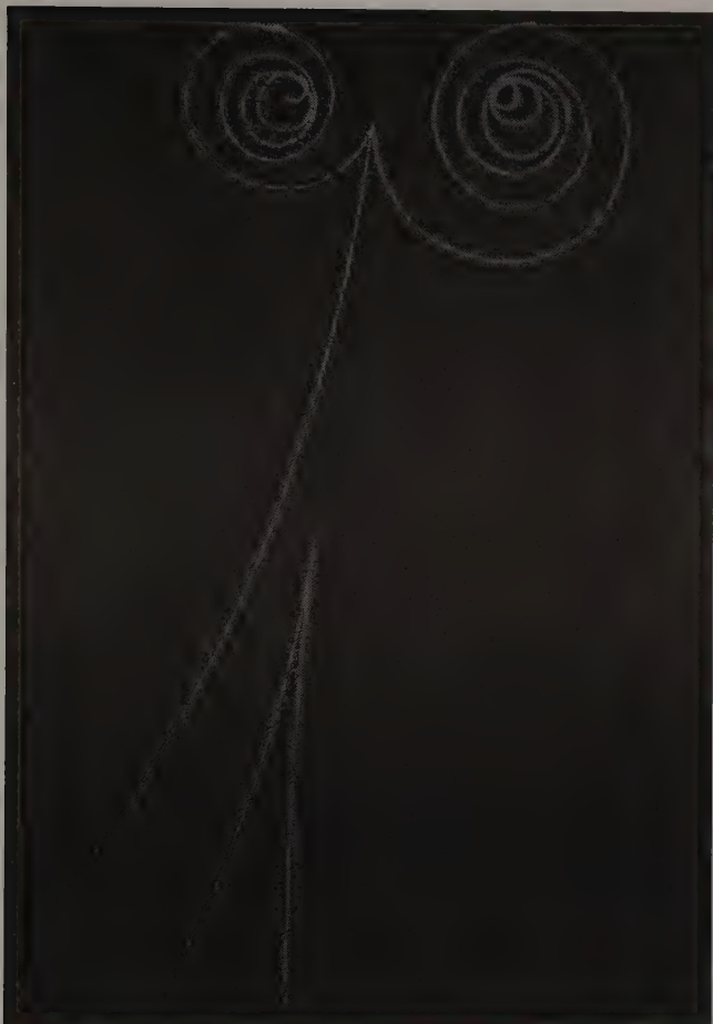
Fig. 11.2 Trails left in a particle detector by an electron and positron. They spiral in opposite directions, hinting at their subtle symmetry. (For more images of positrons see The Particle Explosion by Close, Marten, and Sutton published by Oxford University Press.)
