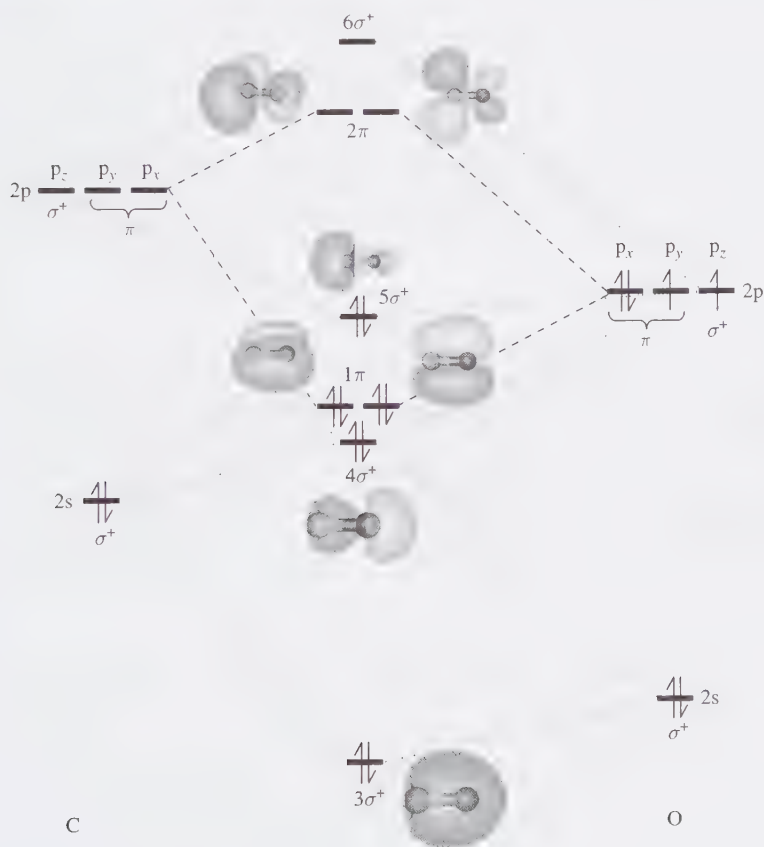
Figure 7.32 The MO diagram for CO.
